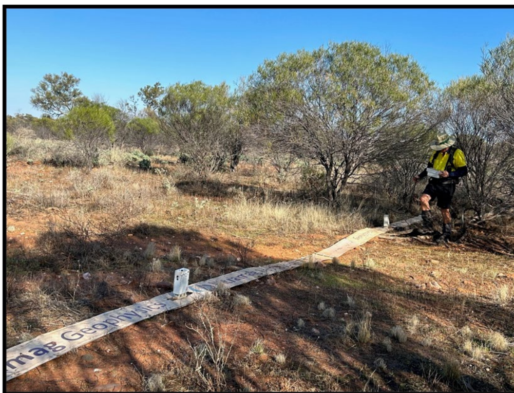
Figure 1: The Deep Ground Penetration Radar equipment at Mt Edon mining lease
