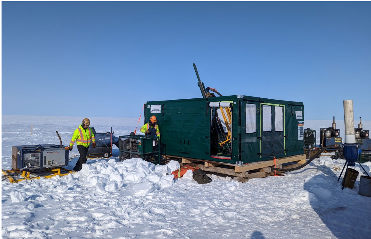
Figure 1: RC drilling underway 4100N Zone, Storm Copper Project. Every drill hole completed to date in the 2023 drill program has successfully intersected copper sulphides.
