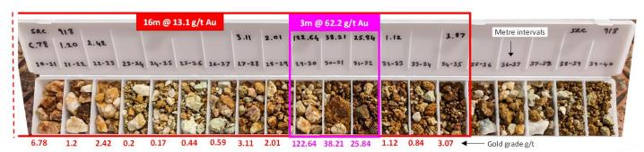
Figure 1: SRC918 chip tray from 20m – 40m showing 15 of the individual metre intervals that returned 16m at 13.1 g/t from 19m gold including the three metre intervals that returned 3m @ 62.2 g/t gold from 30m.
