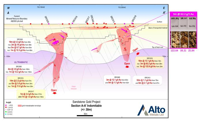
Figure 4: Indomitable Cross section A – A' showing SRC916, SRC917 and SRC918
