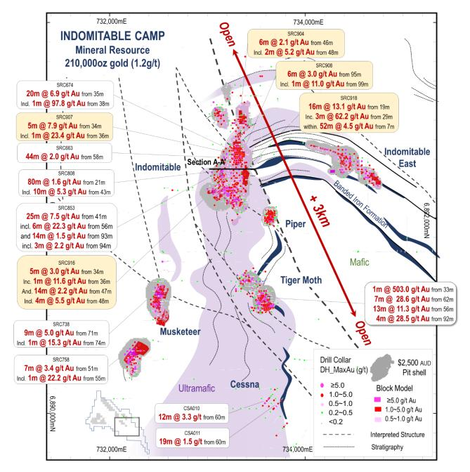
Figure 2: Plan view showing Indomitable deposits and RC high-grade drill results over a simplified geological interpretation.
