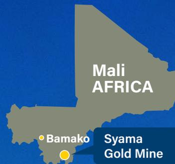
Located in the southwest of Mali, West Africa approximately 30km from the Côte d'Ivoire border and 300km southeast of the capital Bamako, the mine comprises a 2.4Mtpa sulphide processing circuit and a 1.6Mtpa oxide processing circuit.
