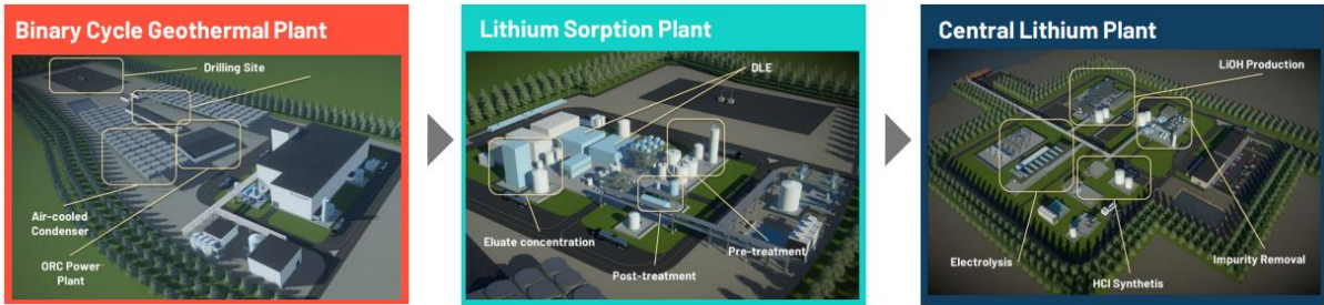
Figure 11.1: Overview of Phase One Project Plants
