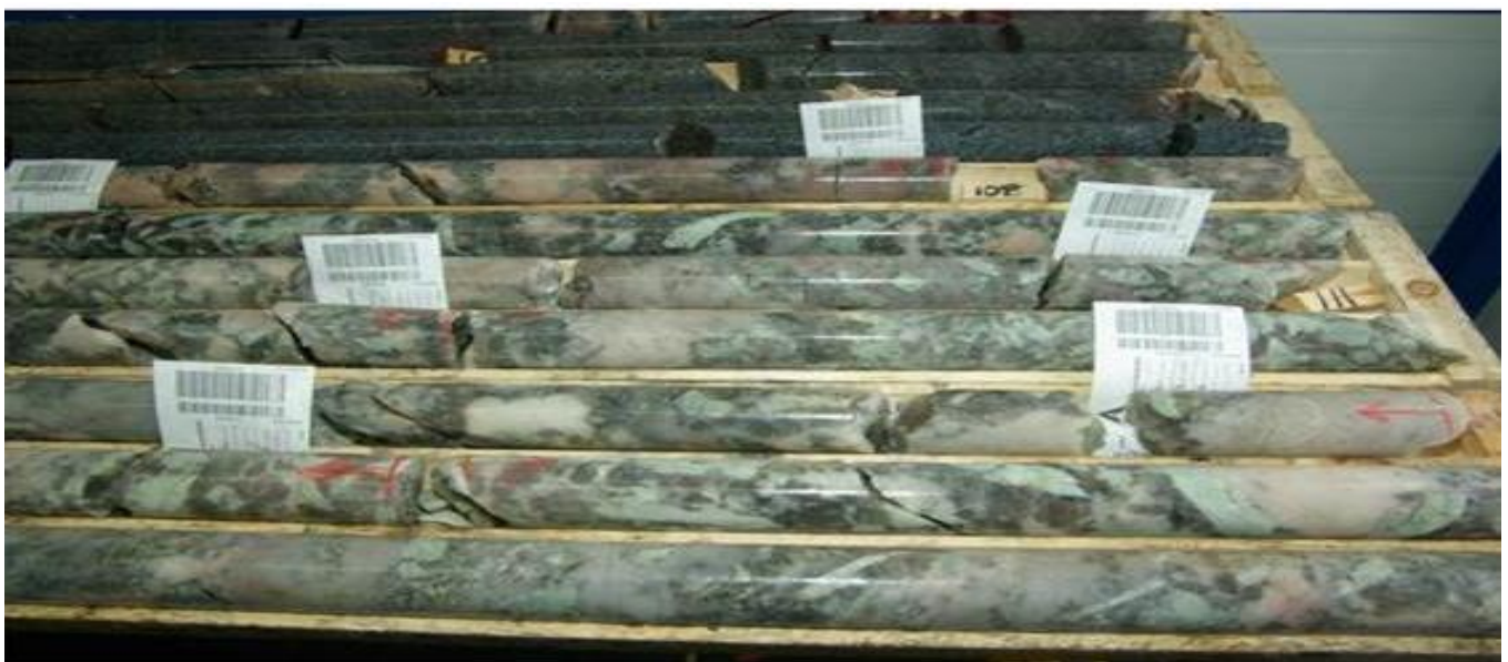
Photo 2: Historical diamond core samples from Main Dyke showing large crystal structure of the spodumene-bearing pegmatites - 12m at 1.57% Li 2 O from 108m in 21-CH-15 7
