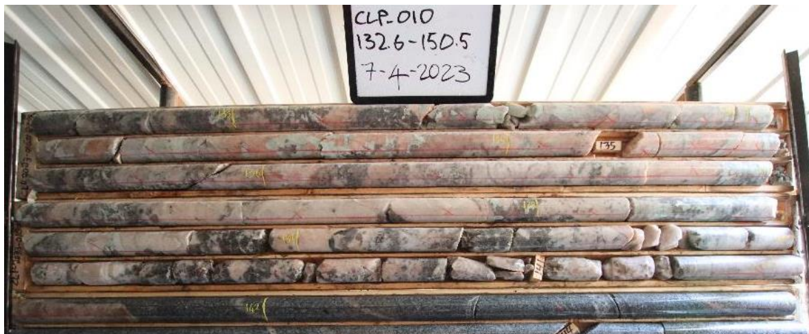
Photo 6: Chubb diamond drill hole CLP010 which intercepted 12.27m of large crystal structure of the spodumene-bearing pegmatites from 129m depth with an estimated 15 to 25% spodumene content.
