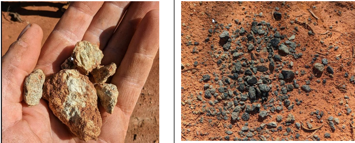
Figure 2 Drill Cuttings located by WXY geologists at BHP AC hole HWAC12 with 45m @ 0.55% Ni
