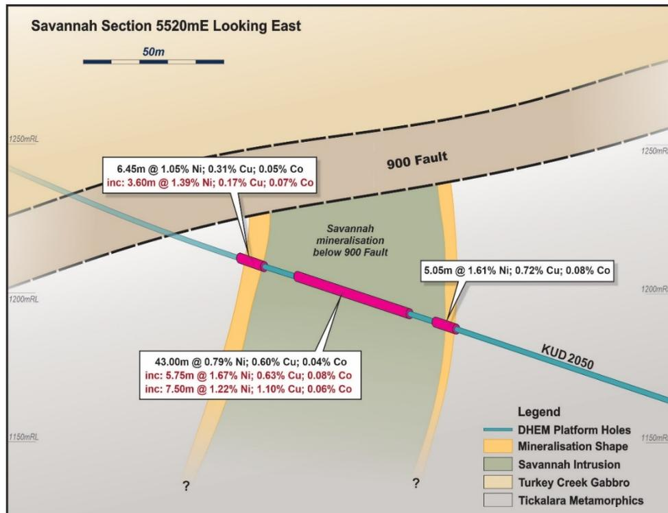
Figure 3: Section 5520E of KUD2050 through the Savannah intrusion and mineralisation below the 900 Fault
