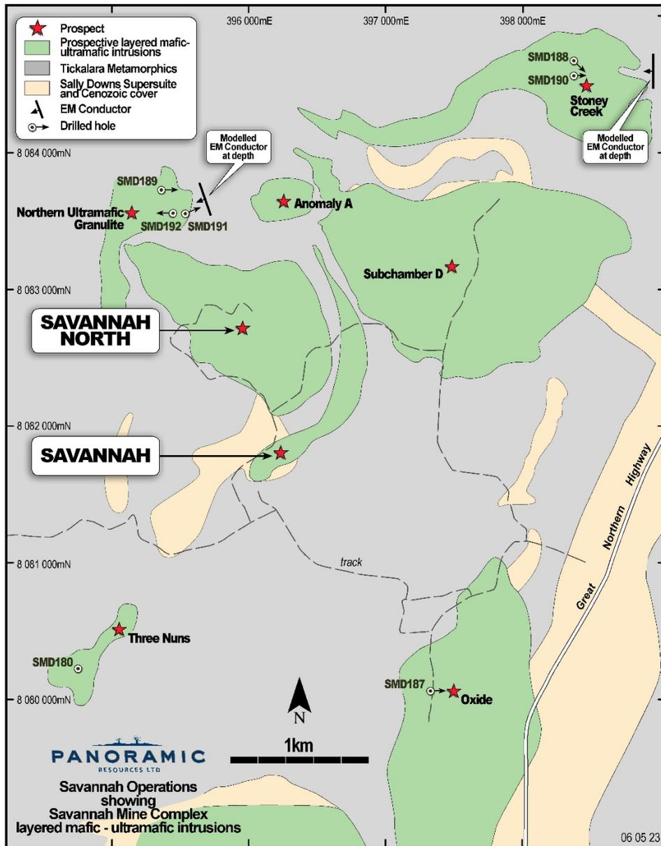
**Figure 4: Plan showing Savannah area intrusions with surface hole locations for DHEM surveying**
