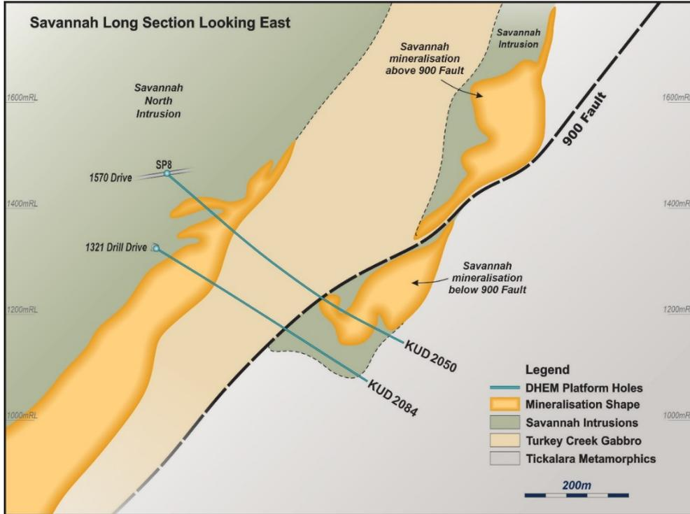
Figure 2: Long section of DHEM platform holes targeting Savannah below the 900 Fault
