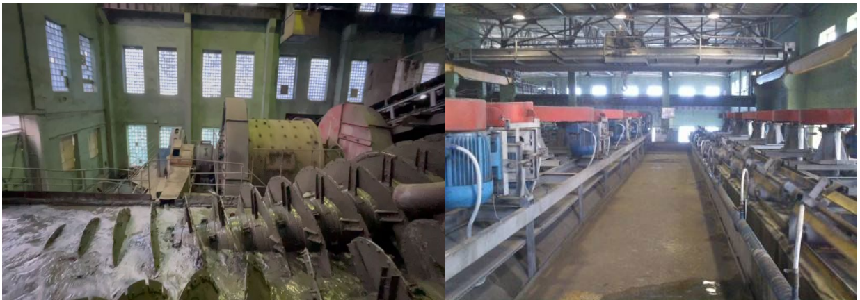
Figure 2 – Grinding, Classification and Flotation of Graphite Ore at the Zavalievsky Concentrator, April 2023
