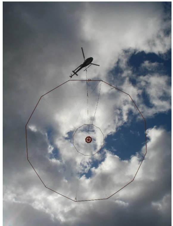
Plate 1: Photo of helicopter VTEM survey
