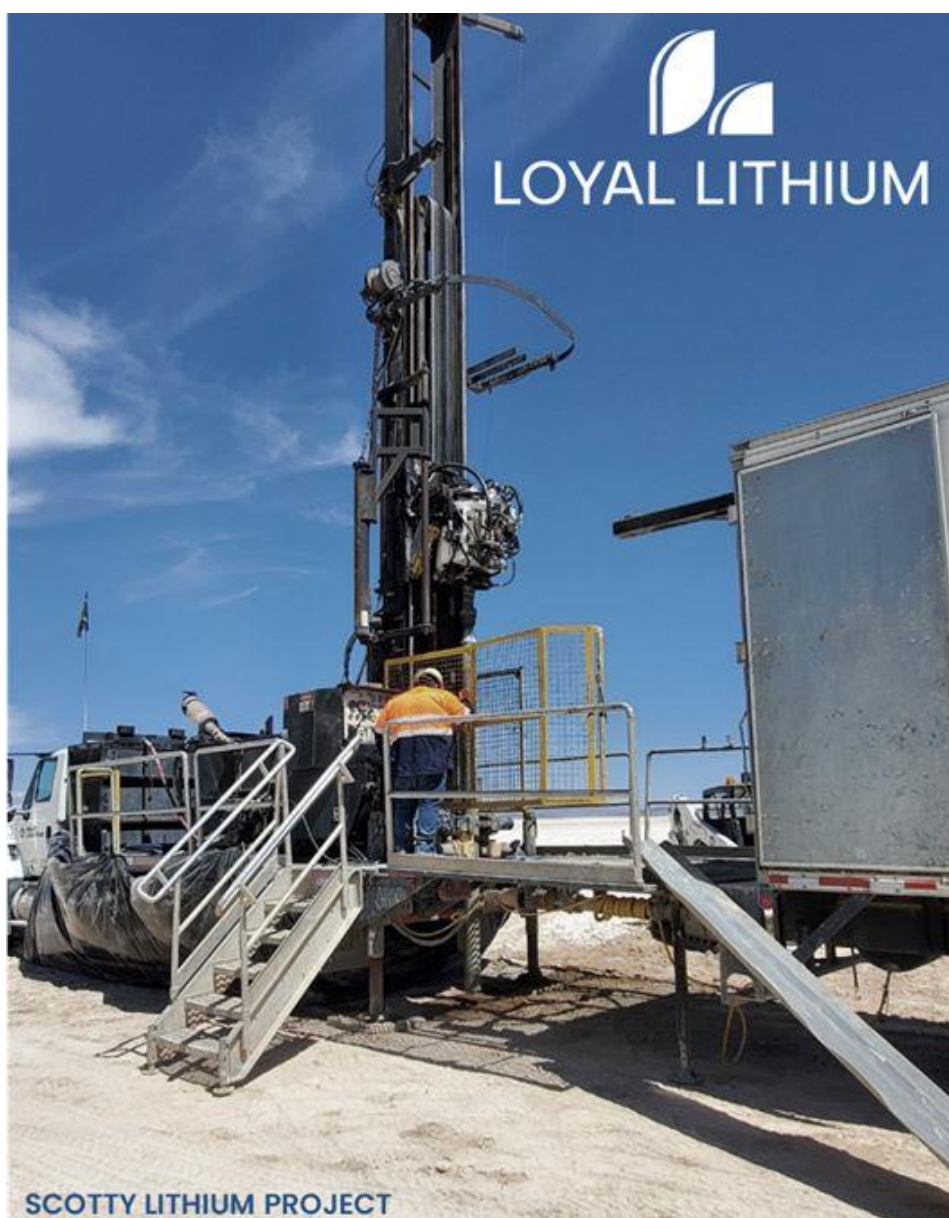
Figure 1: Drill contractor Boart Longyear’ Sonic Drill Rig operating at the Scotty Lithium Project
