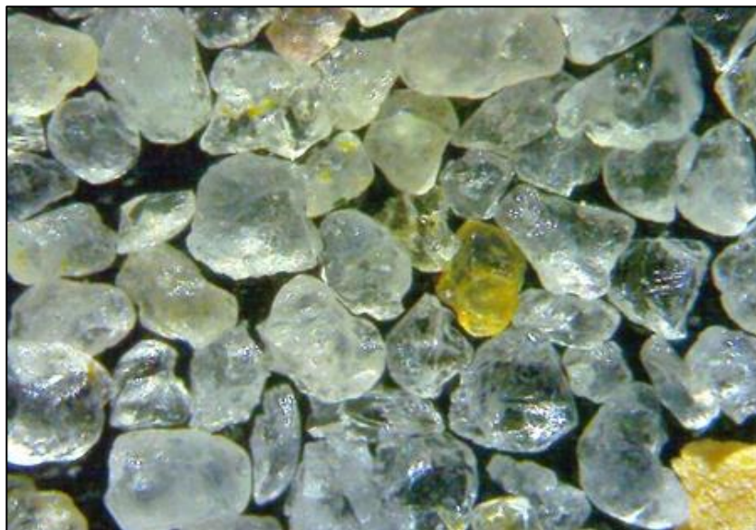
Photomicrograph of VRX 'AFS55' foundry sand product, showing sub-rounded quartz grains
