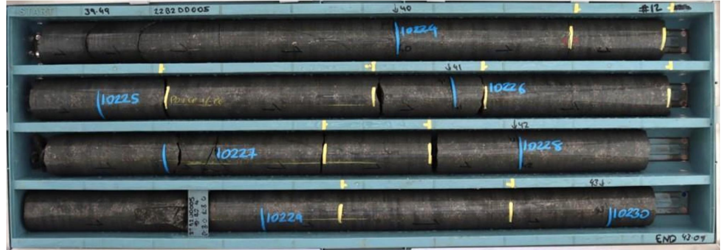
22B2DD005 (38-45.05m – HQ core 61.1mm diameter) incl. 2.0m @ 3.14% Ni_Eq from 41.5m Strongly mineralised dolerite with coarse disseminated angular blebs of fine-grained pyrrhotite, chalcopyrite and pentlandite.
