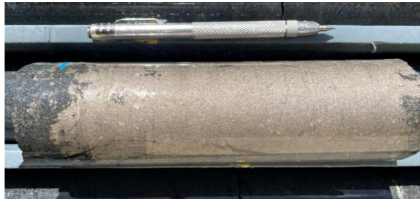
22B2DD006 (86.7-87.0m interval – NQ core 47.6mm diameter) 0.3m @ 2.98% Ni_Eq Strongly mineralised serpentinised ultramafic rock (pyroxenite) with fine-grained massive pyrrhotite with coarse minerals of pentlandite.
