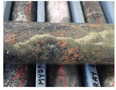
Strongly mineralised breccia zone with chalcopyrite-epidote matrix infill from 23MYDD422 at 378m. This core forms a portion of a zone grading **95m at 0.55% Cu & 0.07g/t Au** (ASX MAG 22 February 2023).
