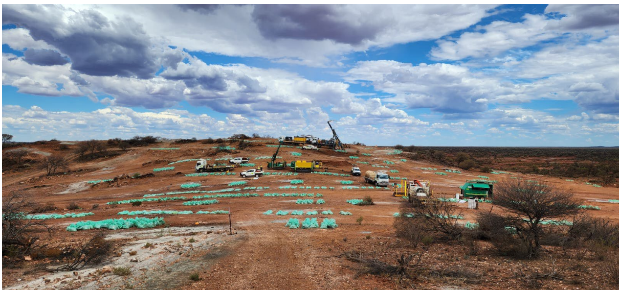
Plate 1 – Apollo Hill gold system – grade control RC and metallurgical diamond drilling at Apollo Hill Bulk Sample Pit Location – early 2023
