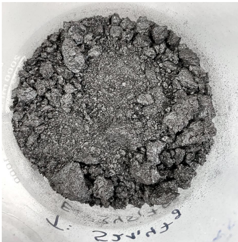
Figure 1: Purified graphitic material produced as part of the ANZAPLAN test work program
