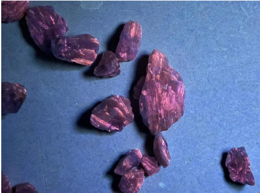
Hole HYRC006 160m – 166m showing pegmatite intercept containing spodumene crystals
