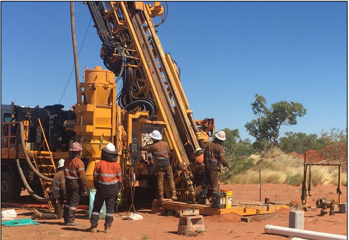
Image 2: DDH1 multi-purpose drilling rig on Stage 3 RC/diamond hole BBDD0026
