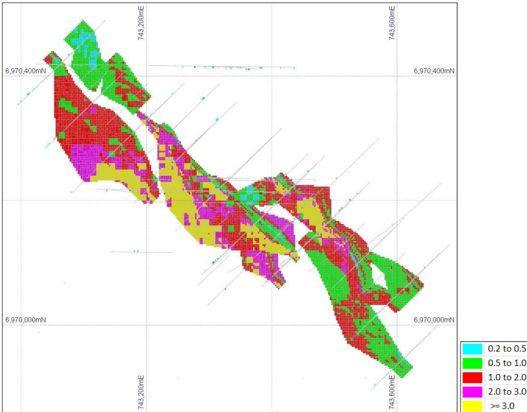
Figure 25: Heron drill hole plan and OK resource block model coloured by Au (g/t)
