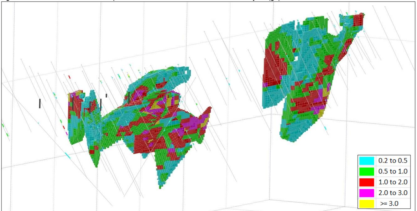
Figure 22: Melbourne Bitter 3D view looking down to the north-west showing drill holes, historic shafts, and OK block model coloured by Au (g/t)
