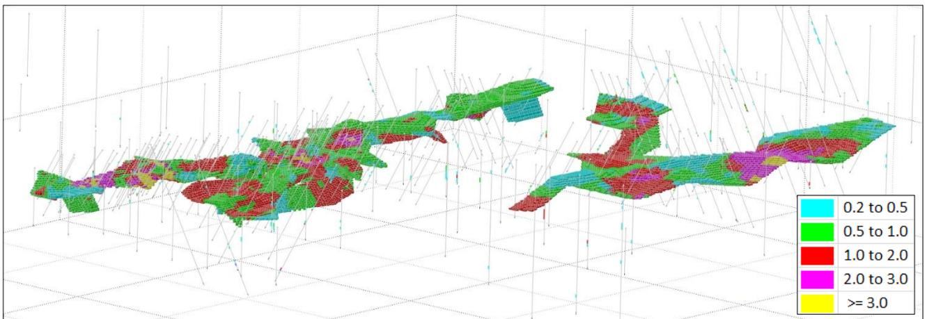
Figure 20: Hyperno-Reliance 3D view looking down to the north-west showing drill holes and OK block model coloured by Au (g/t)
