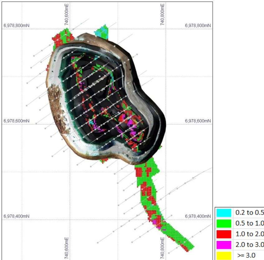
Figure 23: Hawk drill hole plan and OK resource block model coloured by Au (g/t)
