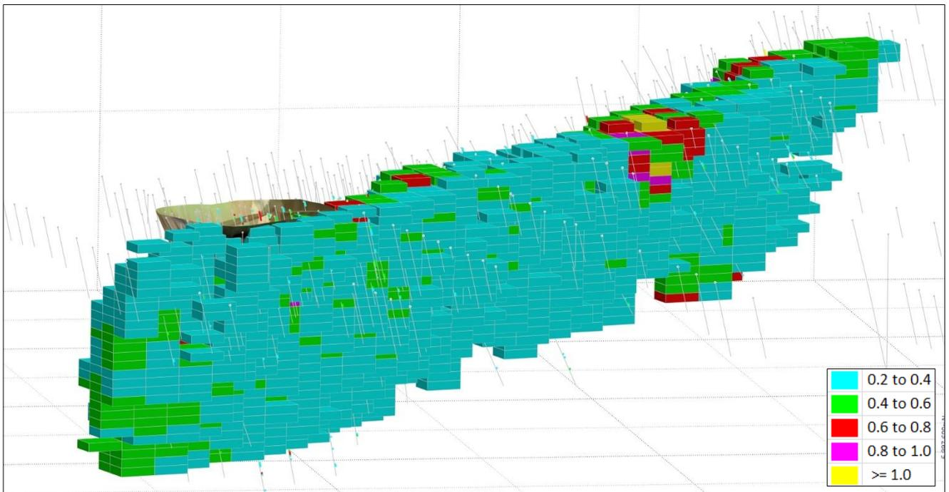
Figure 6: Shiraz 3D view looking down to the north-west showing drill holes and MIK block model coloured by E type panel Au grade (g/t).
