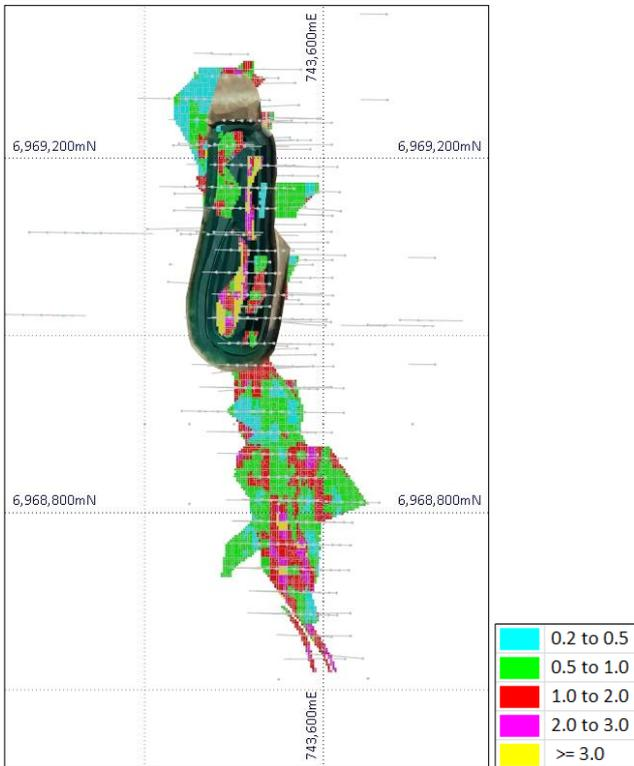
Figure 27: Heron South drill hole plan and OK resource block model coloured by Au (g/t)
