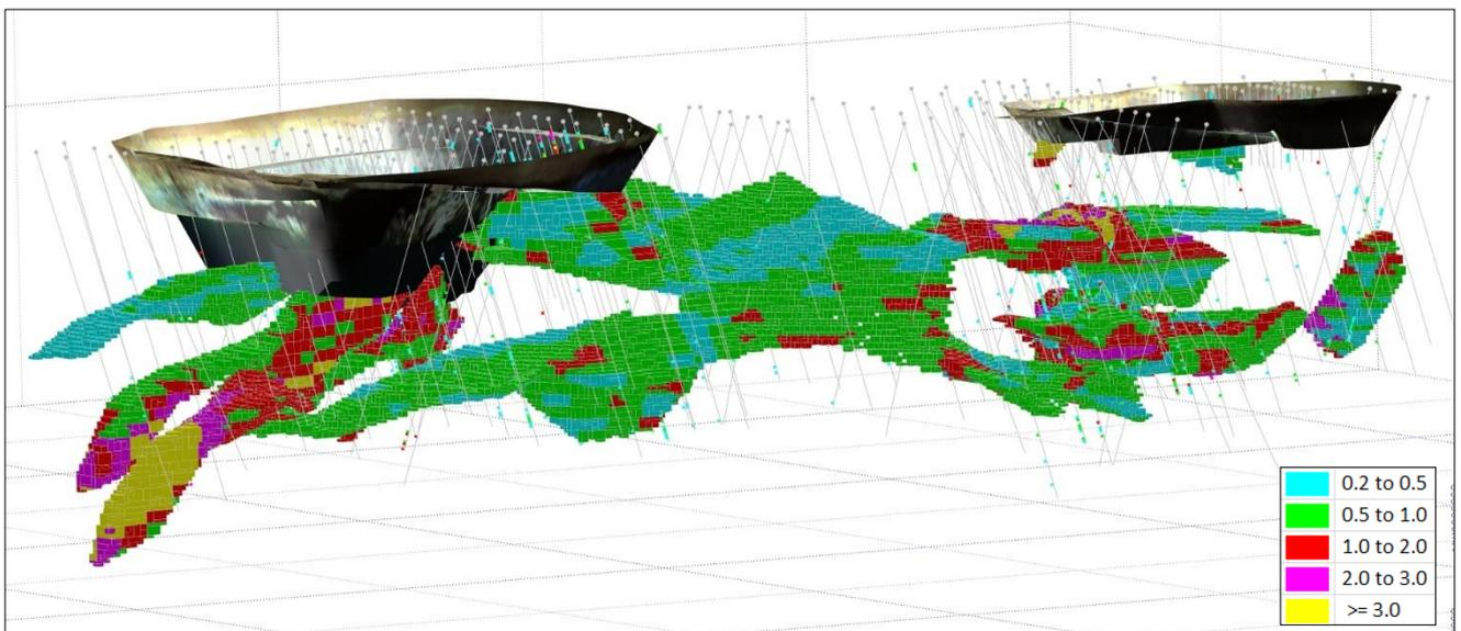
Figure 32: Wedge 3D looking down to the north-west showing drill holes and OK block model coloured by Au (g/t)
