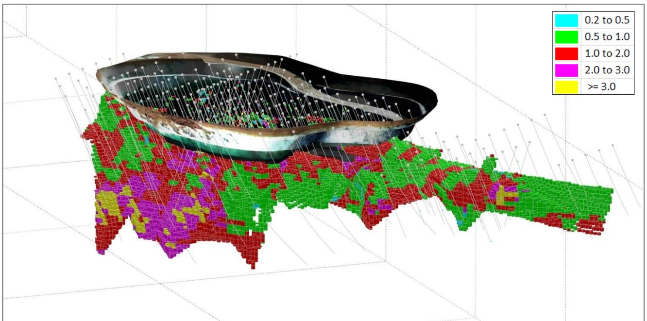
Figure 24: Hawk 3D looking down to the north-east showing drill holes and OK block model coloured by Au (g/t)
