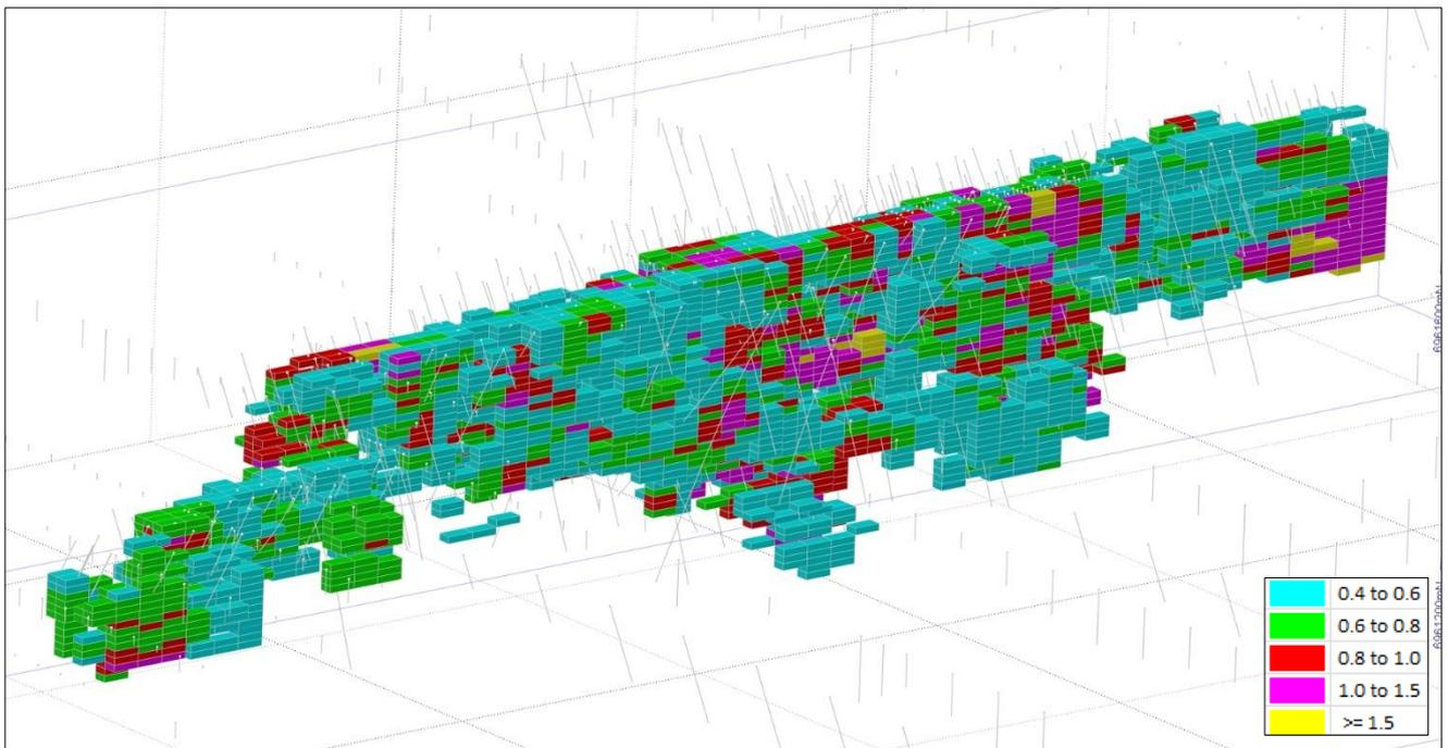
Figure 4: Howards 3D view looking down to the north-west showing drill holes and MIK block model coloured by E type panel Au grade (g/t)
