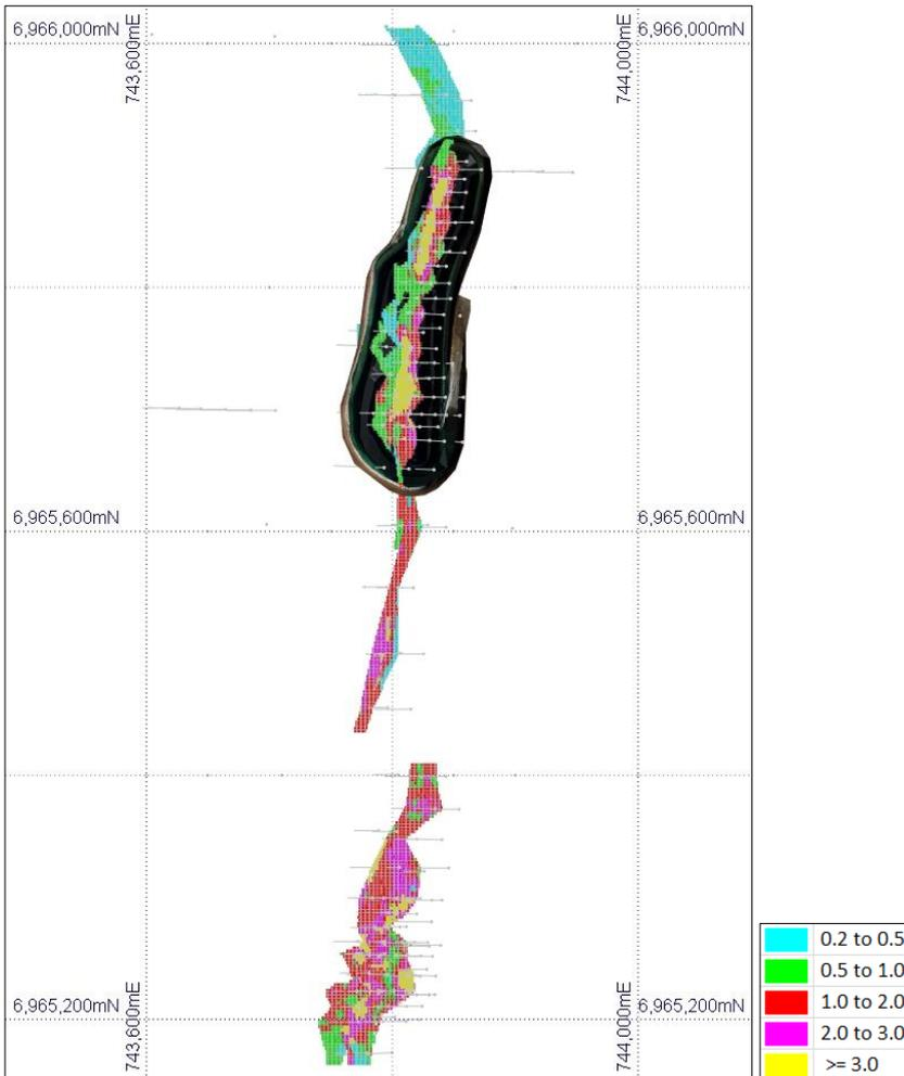
Figure 7: Deep South Reliance drill hole plan and OK resource block model coloured by Au (g/t)
