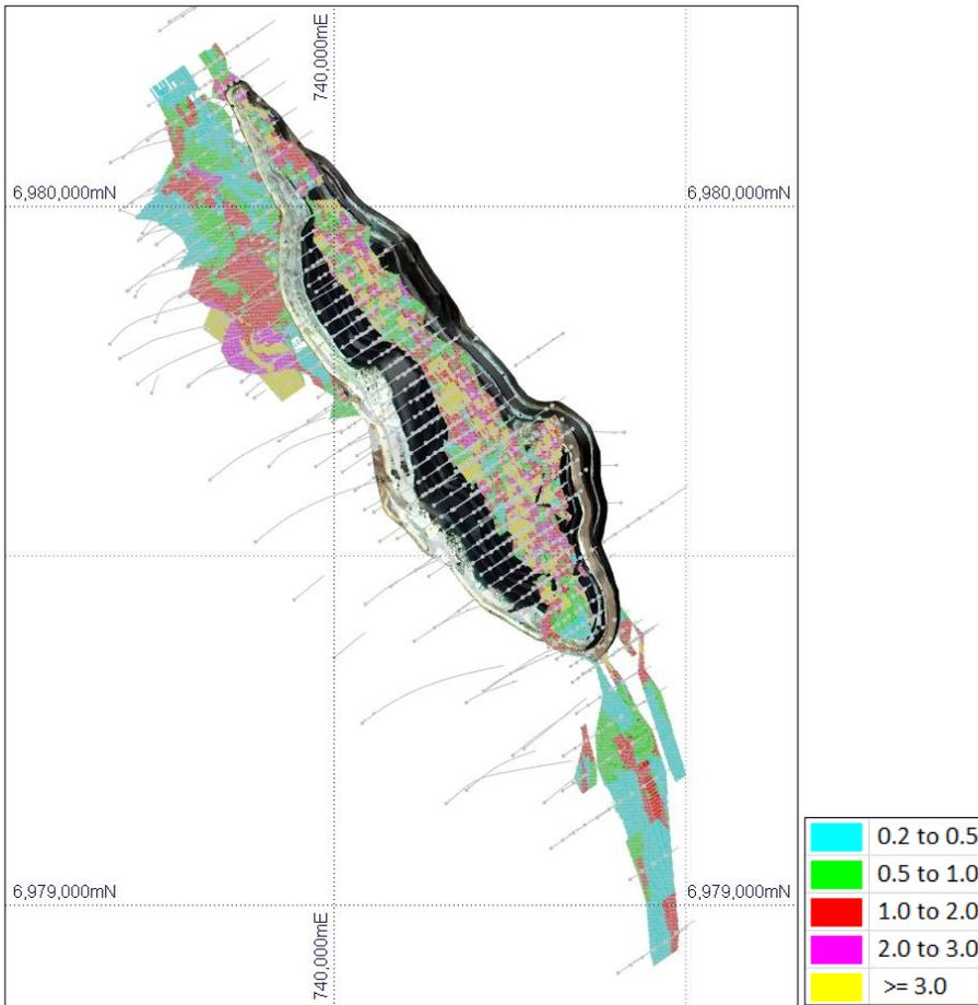
Figure 17: Kingfisher drill hole plan and OK resource block model coloured by Au (g/t)
