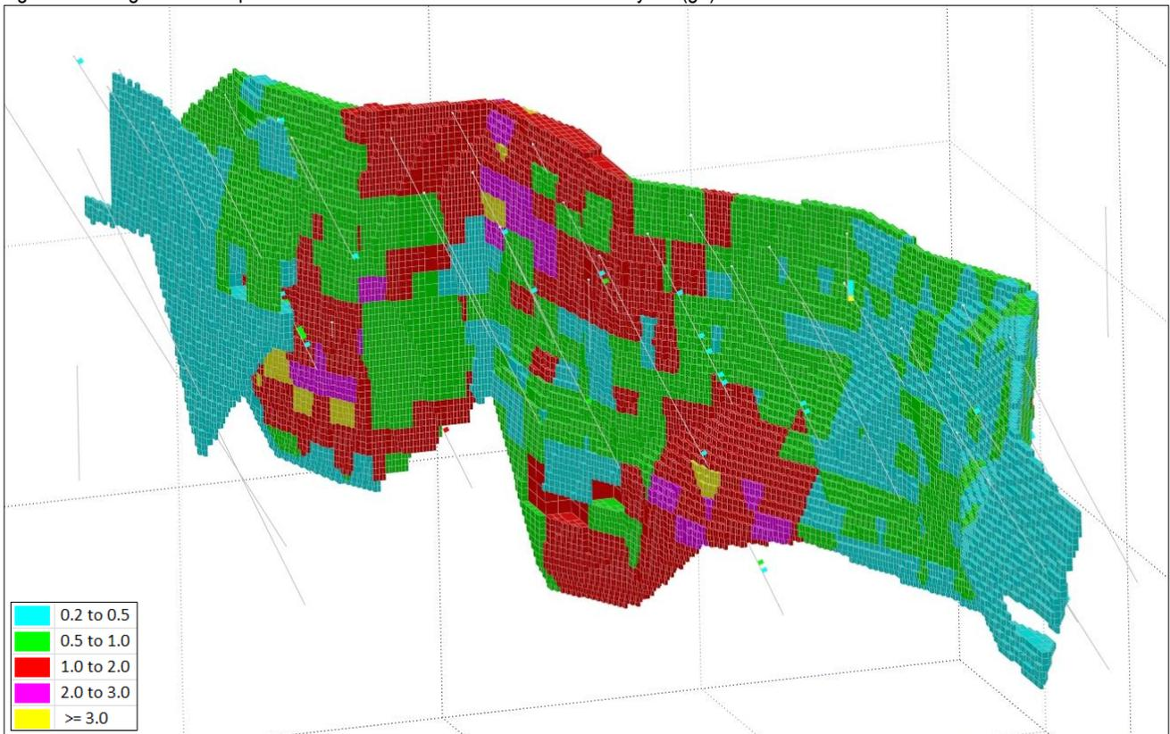
Figure 14: Fangio 3D view looking down to the north-east showing drill holes and OK block model coloured by Au (g/t)
