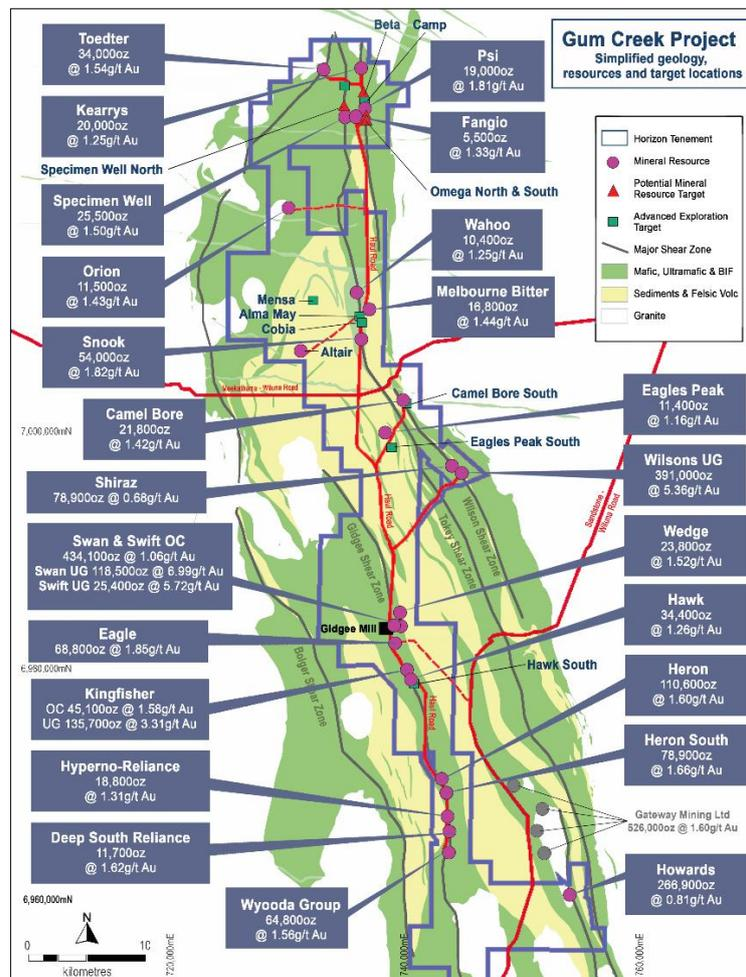
Figure 2: Gum Creek Gold Project Mineral Resources, Advanced Mineral Resource Targets and Exploration Targets over simplified geology<sup>3</sup>
