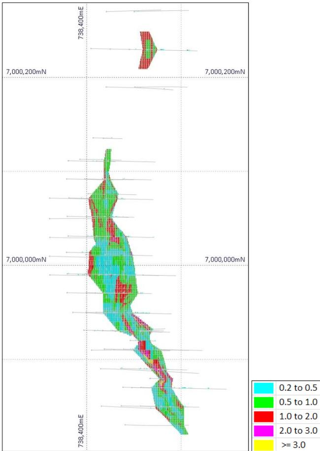
Figure 11: Eagles Peak drill hole plan and OK resource block model coloured by Au (g/t)
