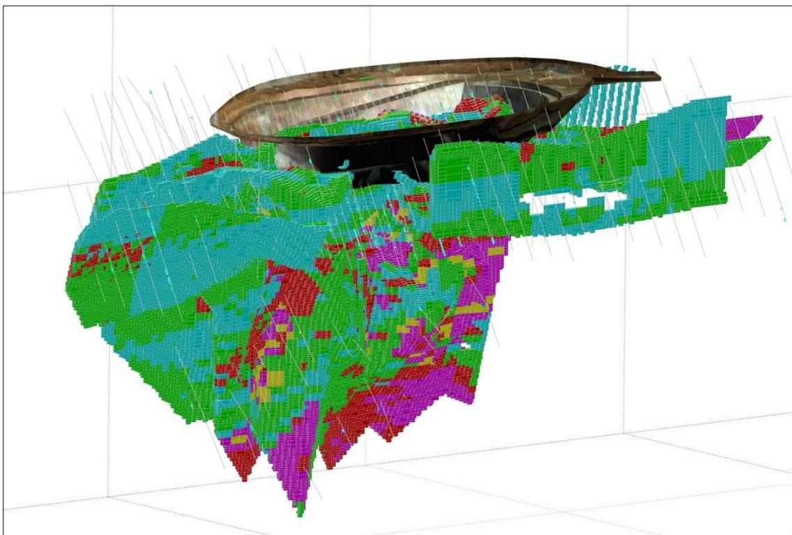
Figure 10: Eagle 3D view looking down to the north-west showing drill holes and OK block model coloured by Au (g/t)
