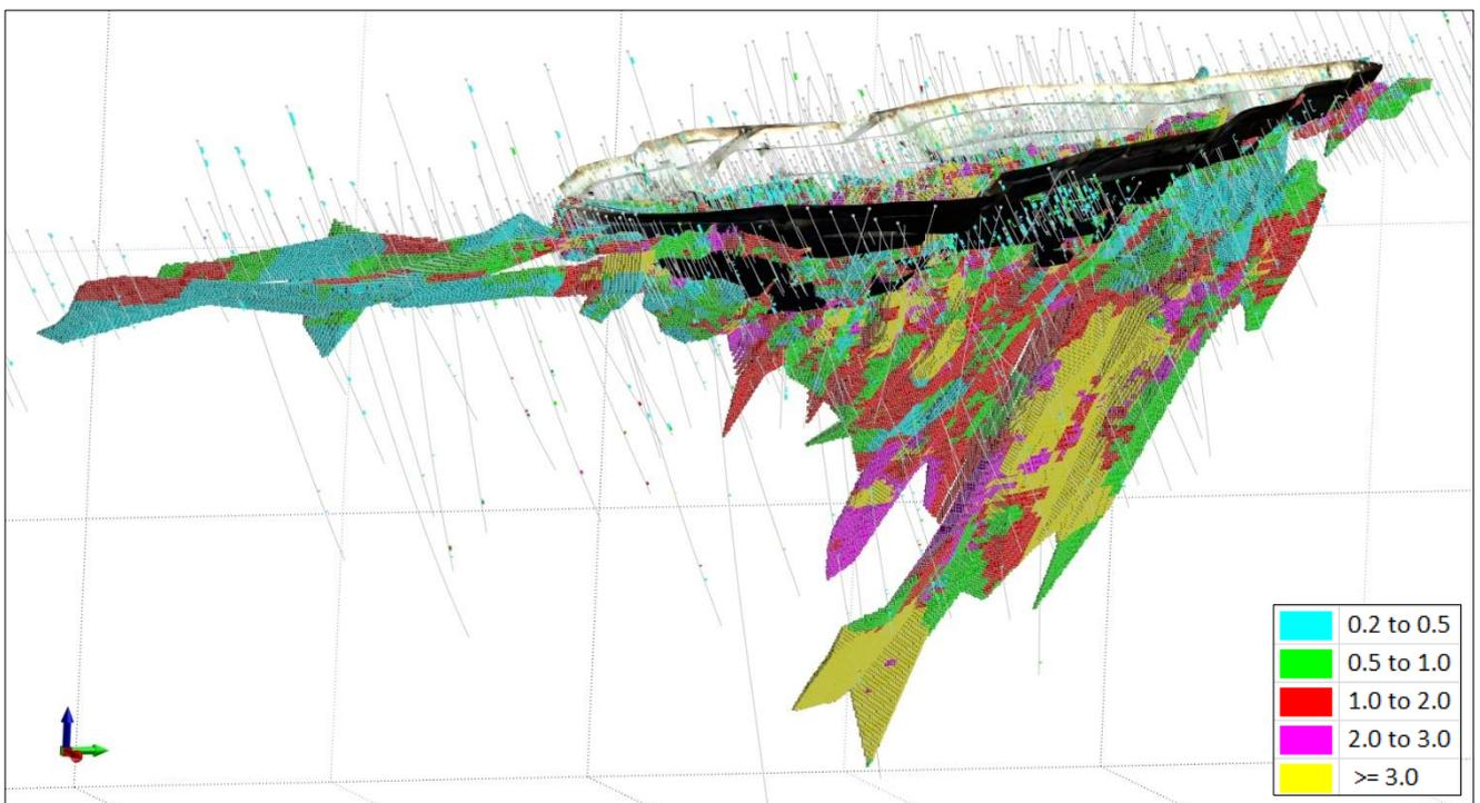
Figure 18: Kingfisher 3D view looking down to the north-west showing drill holes and OK block model coloured by Au (g/t)
