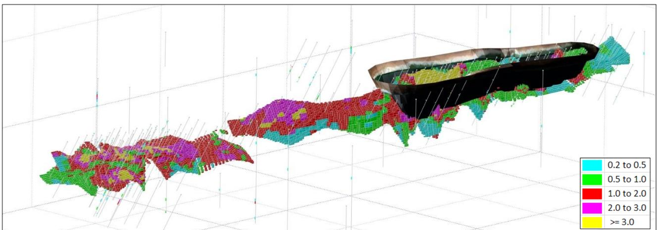
Figure 8: Deep South Reliance 3D view looking down to the north-west showing drill holes and OK block model coloured by Au (g/t)
