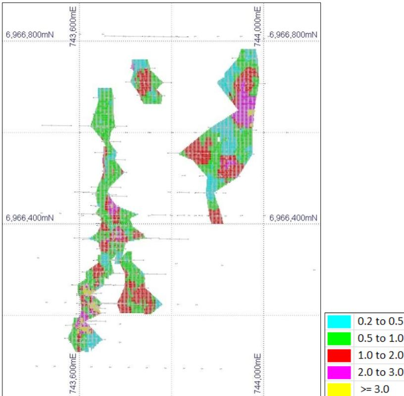
Figure 19: Hyperno-Reliance drill hole plan and OK resource block model coloured by Au (g/t)
