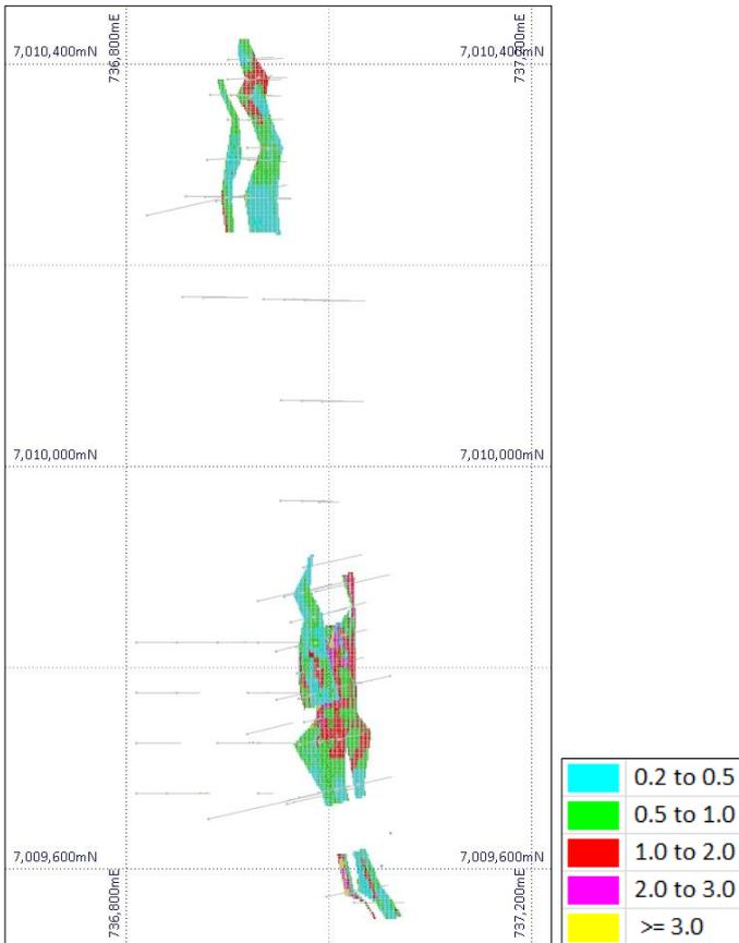
Figure 21: Melbourne Bitter drill hole plan and OK resource block model coloured by Au (g/t)
