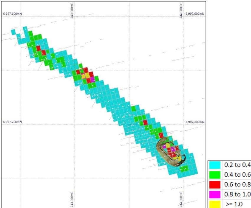
Figure 5: Shiraz drill hole plan and MIK resource block model coloured by E type panel Au grade (g/t).
