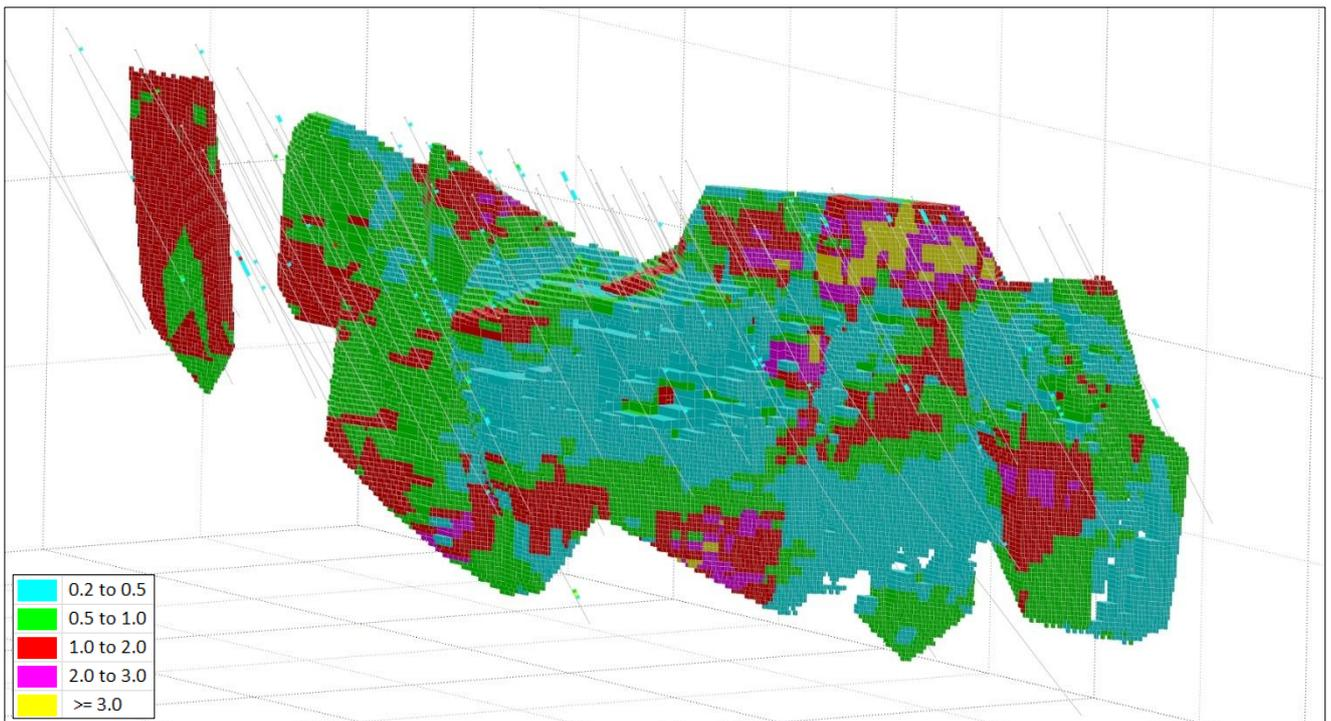
Figure 12: Eagles Peak 3D view looking down to the north-east showing drill holes and OK block model coloured by Au (g/t)
