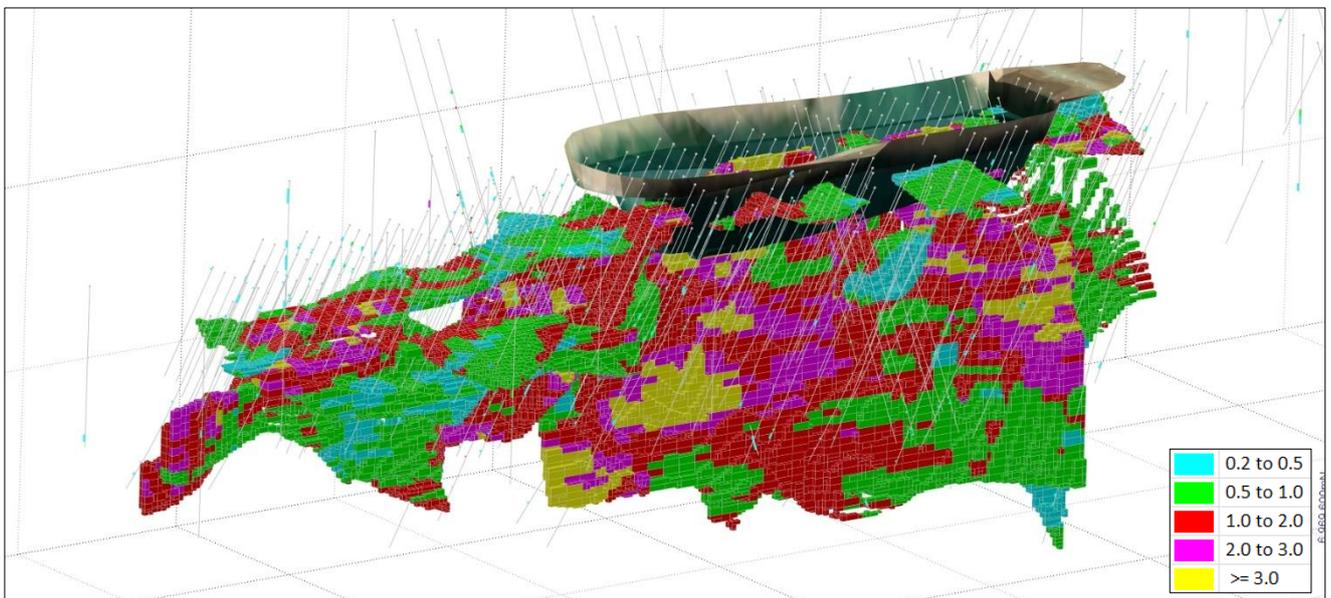
Figure 28: Heron South 3D looking down to the north-west showing drill holes and OK block model coloured by Au (g/t)
