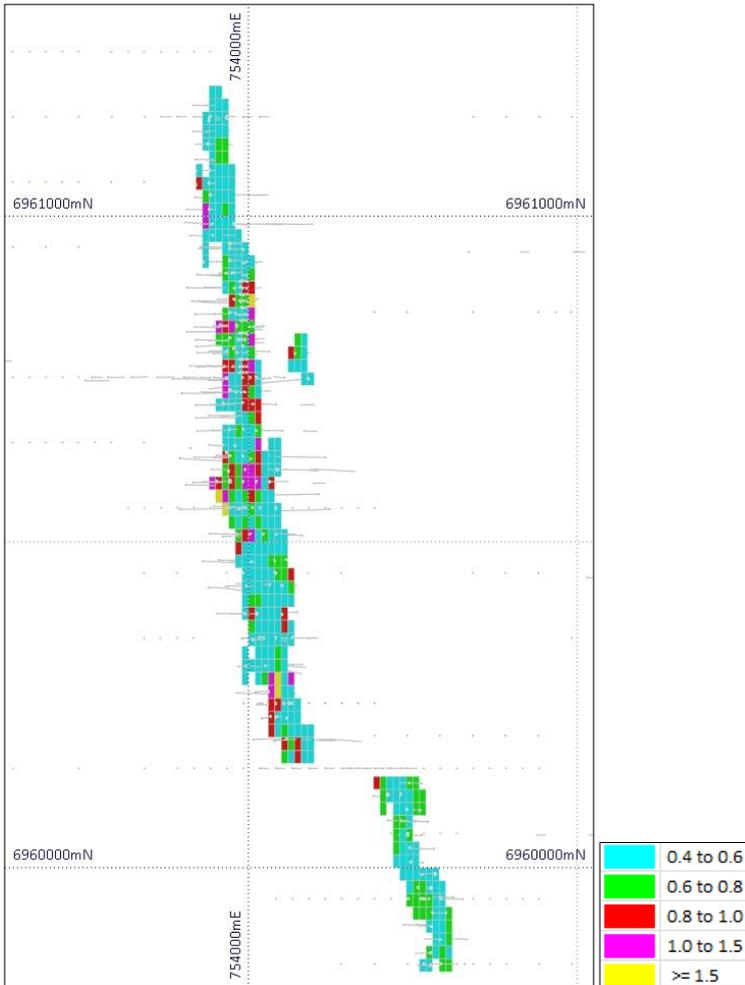
Figure 3: Howards drill hole plan and MIK resource block model coloured by E type panel Au grade (g/t)
