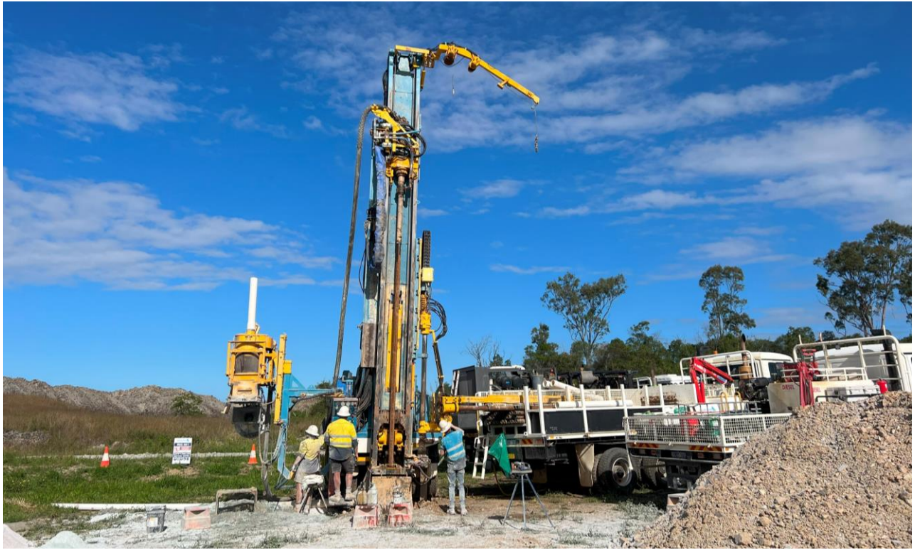
Figure 1: QMines RC drill rig in operation at Mt Chalmers.
