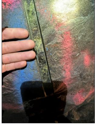
Photos 3 and 4 – Channel cuts undertaken as part of the underground sampling program. Note massive chalcopyrite mineralisation in the cut, hiding behind the surface grime. "The side walls are seemingly unimpressive until we cut into them and reveal the amazing mineralisation hidden under years of grime" notes Director of Exploration, Brian Paull.
