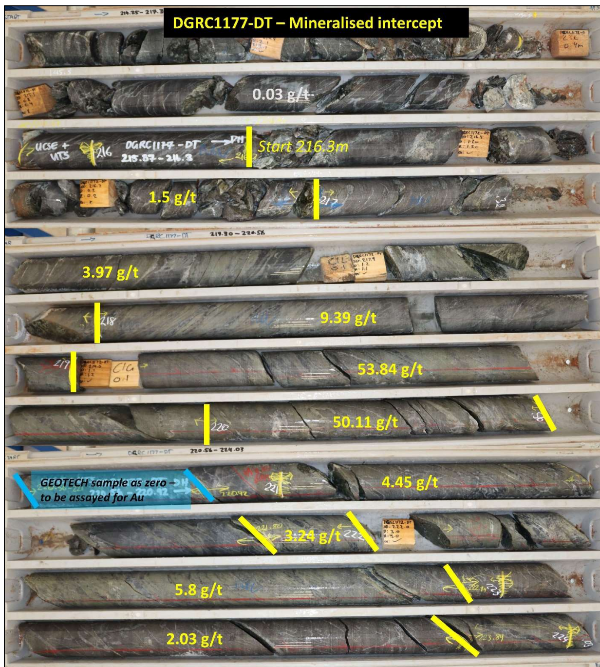
Figure 5: Photographs of drill-core from DGRC1177-DT (15.7m @ 13.51g/t Au) from the Never Never Gold Deposit. Silica “flooding” and sericite/biotite alteration is evident throughout the consistent high-grade mineralisation. Note: two intervals labelled as “GEOTECH” are given a value of 0.00g/t Au for the purposes of calculating the total intercept.
