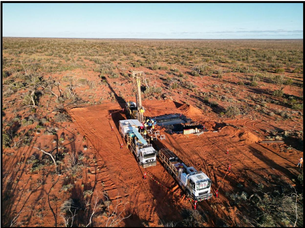
**Photo 1:** Diamond drilling underway at Octagonal at Target Area B.
