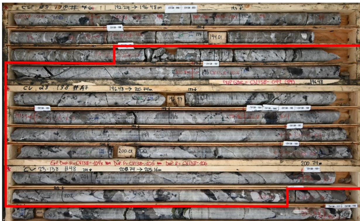
Figure 5: Spodumene pegmatite in drill hole CV23-138 – 8.1 m at 5.01% Li 2 O (red box)
