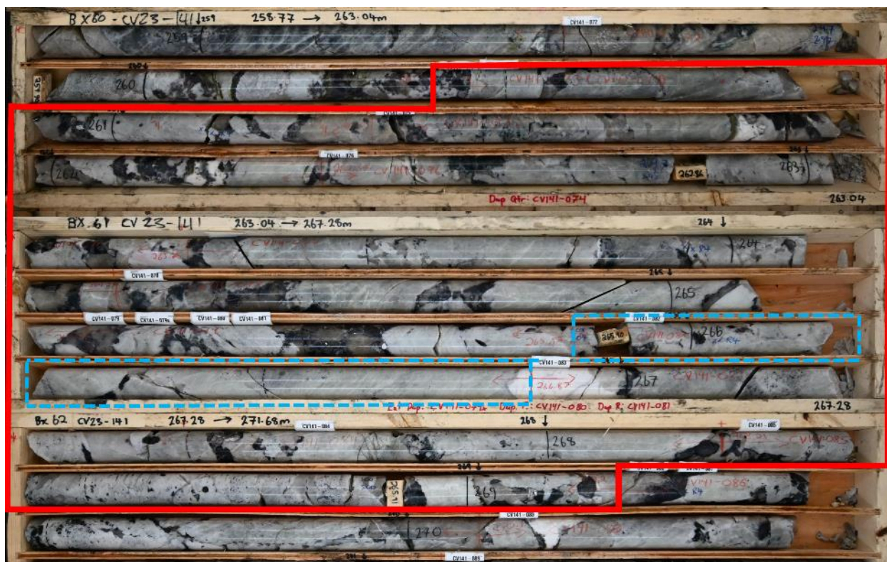
Figure 4: Spodumene pegmatite in drill hole CV23-141 – 8.8 m at 5.20% Li 2 O (red box), including 1.0 m at 6.74% Li 2 O (blue box)
