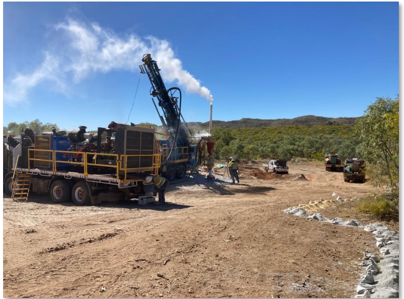
Plate 1: RC drilling in progress at Ardmore
