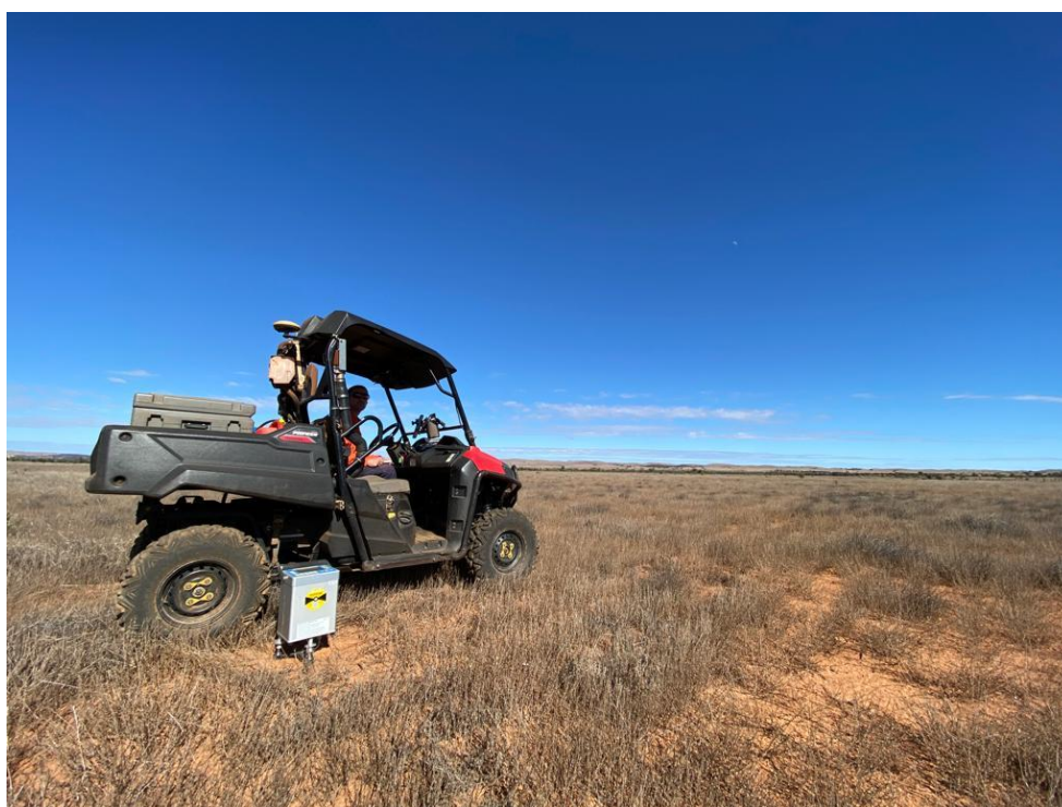
Figure 1. Atlas Geophysics ATV with mounted gravity equipment in the field on Orroroo Project EL6552
