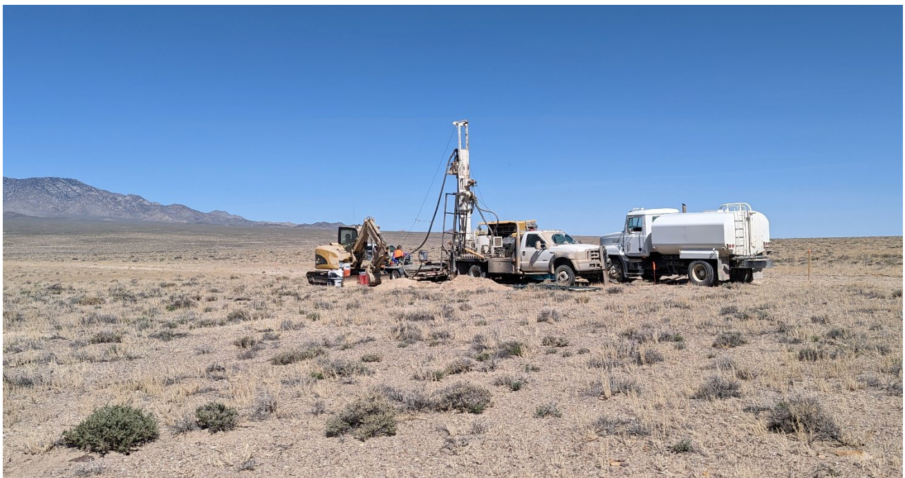
Figure 3. Photograph of air core drill rig set up over drill hole PL04.
