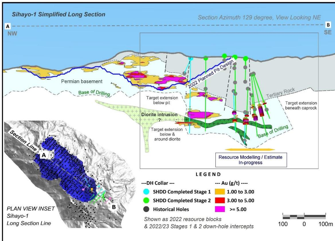
**Figure 7: Long section of Sihayo pit showing beneath pit mineralisation and intercepts from the recent Stage 2 drilling program<sup>9</sup>**
