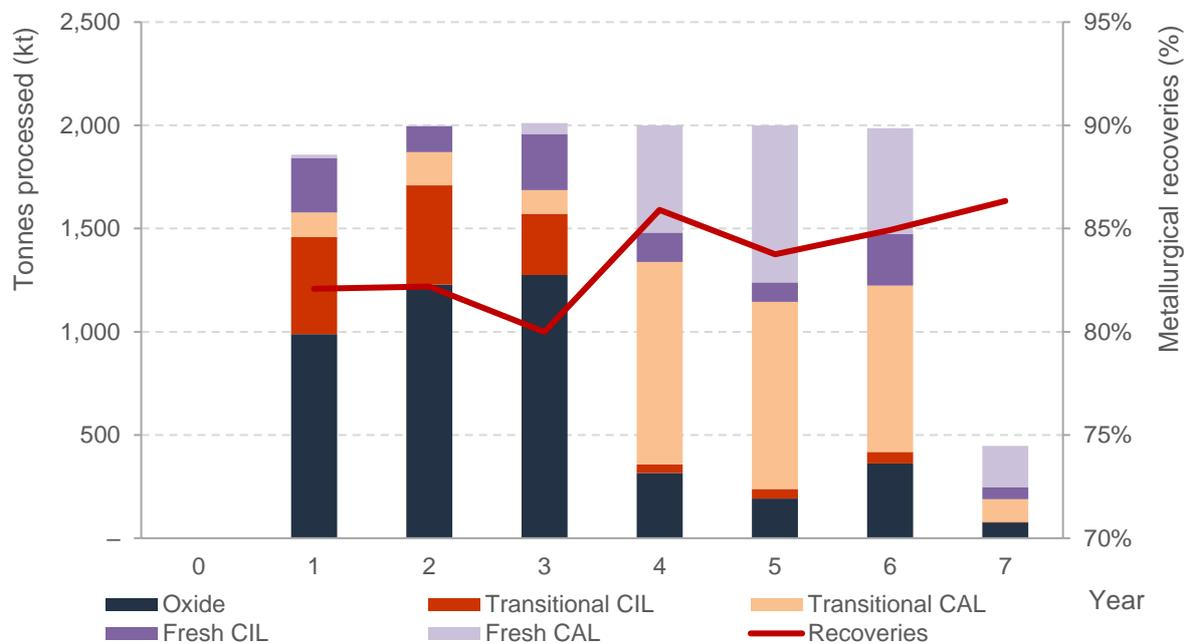
Figure A - 8: Annual processing plant throughput by ore type and head grade
