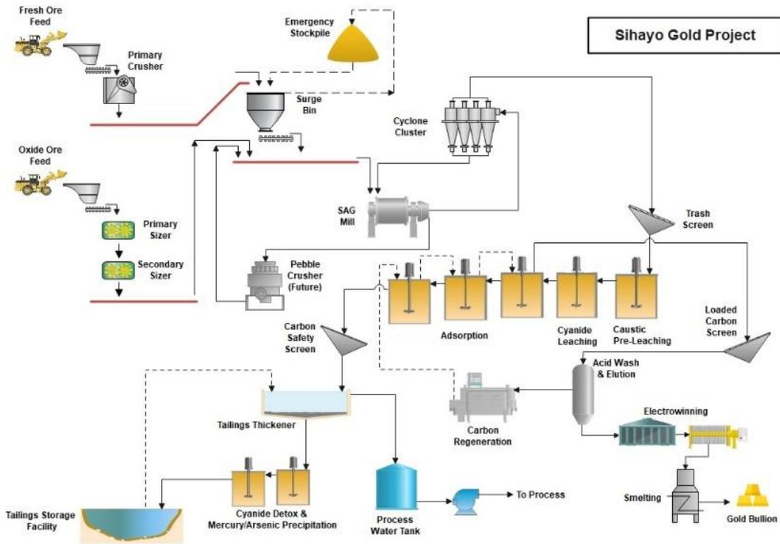
Figure 2: Updated processing flow sheet for the Sihayo Starter Project
