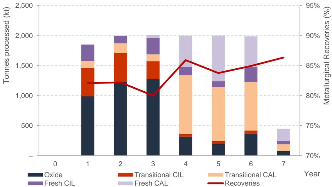
Figure 3: Processing schedule by mineralisation type and processing route
