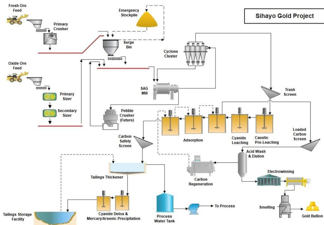
**Figure A - 9: Process flow sheet**
