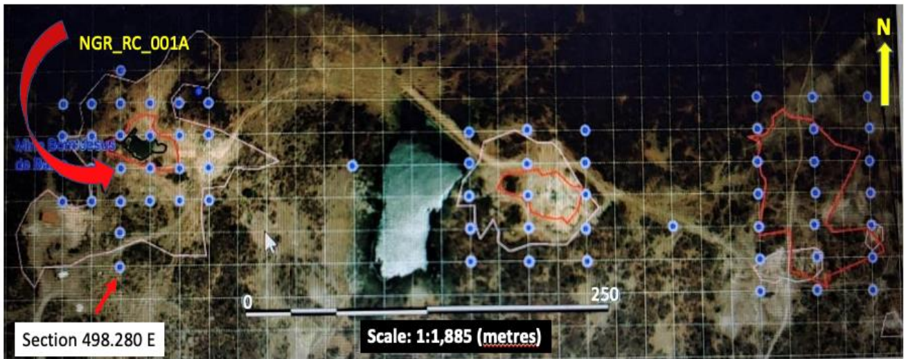
Figure 1: Google Earth image of Mina Bom Jesus de Baixo pit showing the 20m x 20m drill grids (blue dots proposed drill holes) starting in the west with first hole NGR_RC_001A. Drill plan is to move east over the other two (2) outcropping areas (red polygon being pegmatite outcrop; pink polygon being pegmatite rubble).
