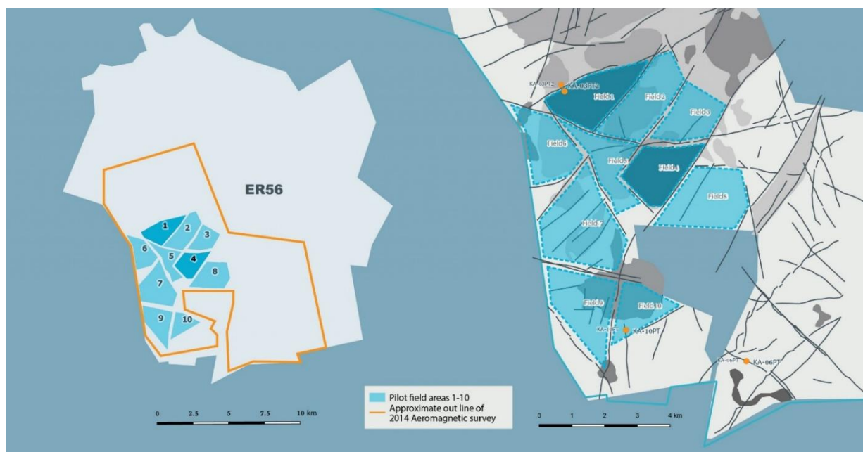
Figure 5-1: Pilot field areas 1-10 (volumetric compartments) interpreted from the 2014 aeromagnetic survey
