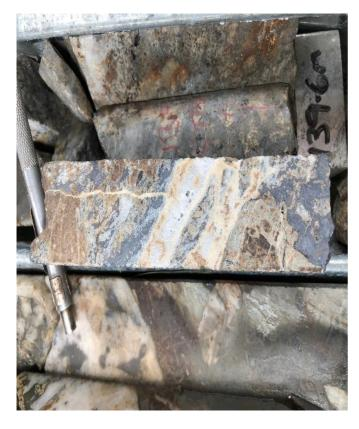
Figure 2 – Drill Hole *RBE055 Massive sulphides with* stockwork quartz carbonate veining. Assay Results 0.6m @ 0.05% Cu, 12.0% Pb; 3.0% Zn; 167g/t Ag from 183.5m
