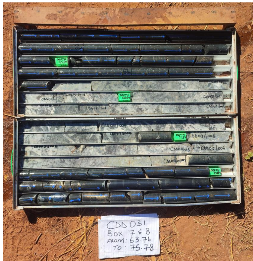
Figure 7: Wide high-grade spodumene mineralised zone in drill hole CDD031 (Pegmatite E)
