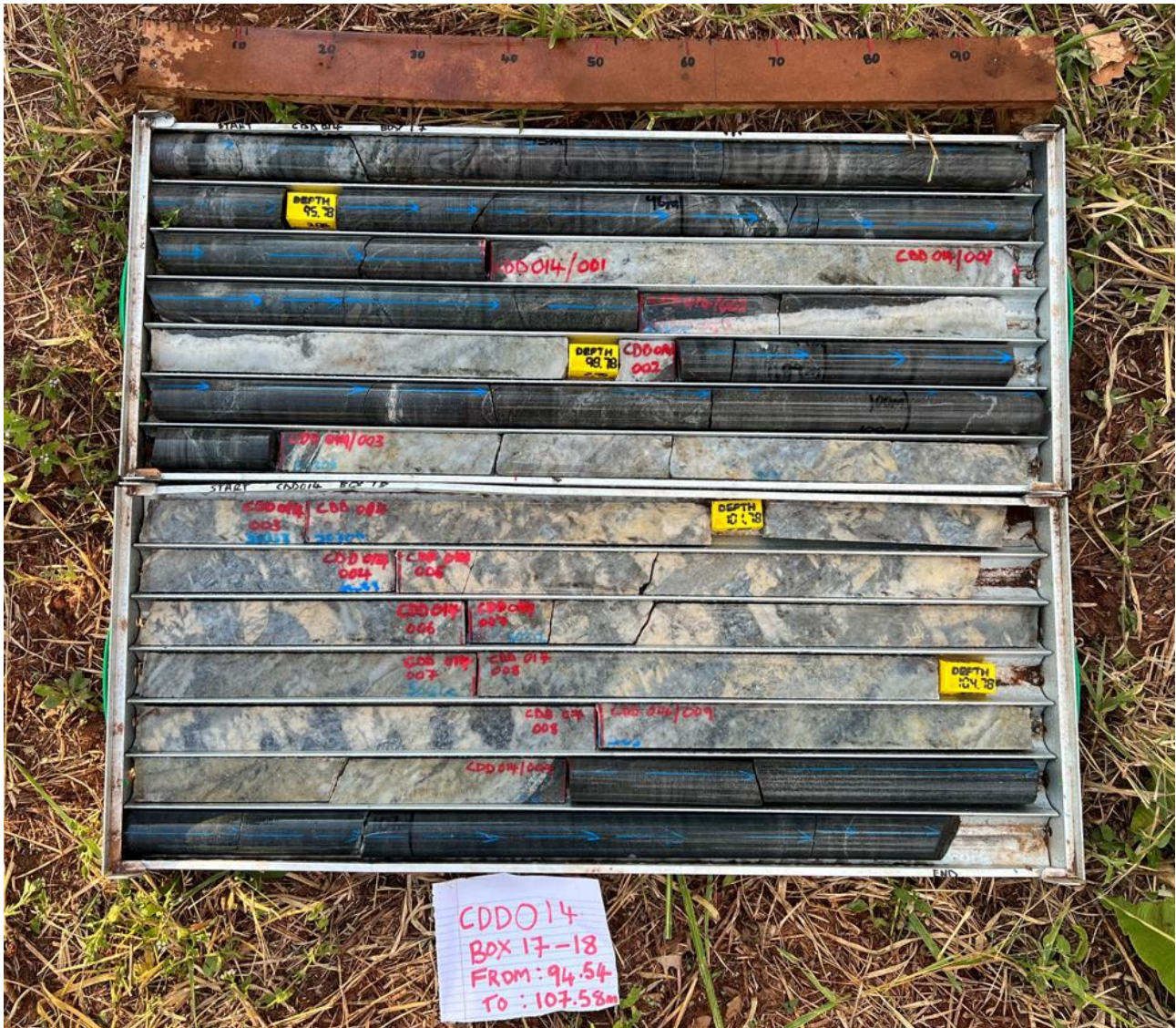
Figure 4: Coarse high-grade spodumene intersected in drill hole CDD014 (Pegmatite D)
