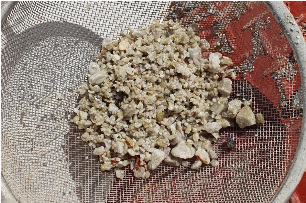
Figure 2 – Sieve showing spodumene from hole MRC082 between 14m-15m
