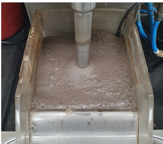
Figure 1: Photo of the third stage floatation which produced a concentrate with 31.22% TREO @ 87.1% TREO recovery and 6.7% mass recovery.
