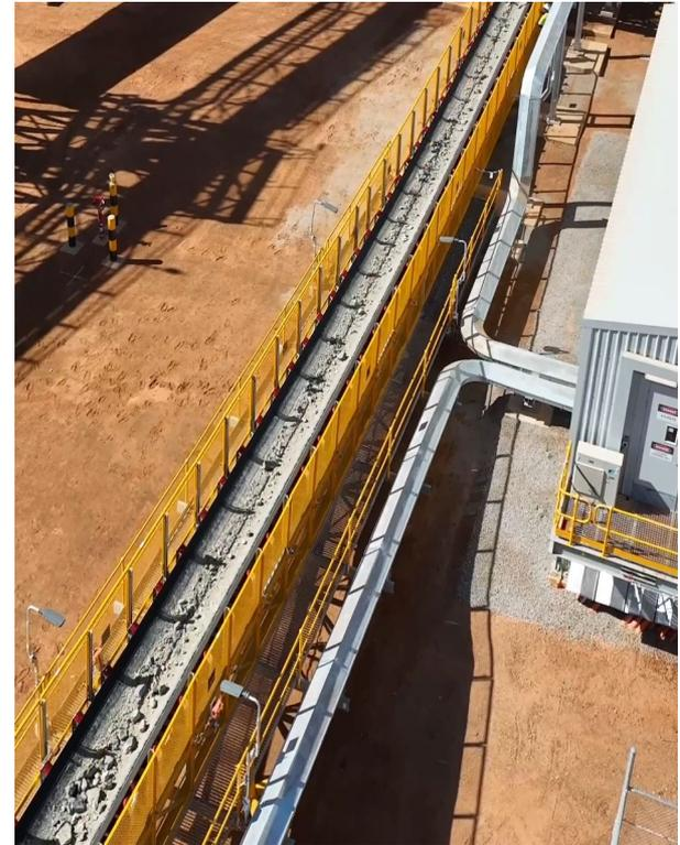
Crushed ore on conveyor belt at Mt Holland.
