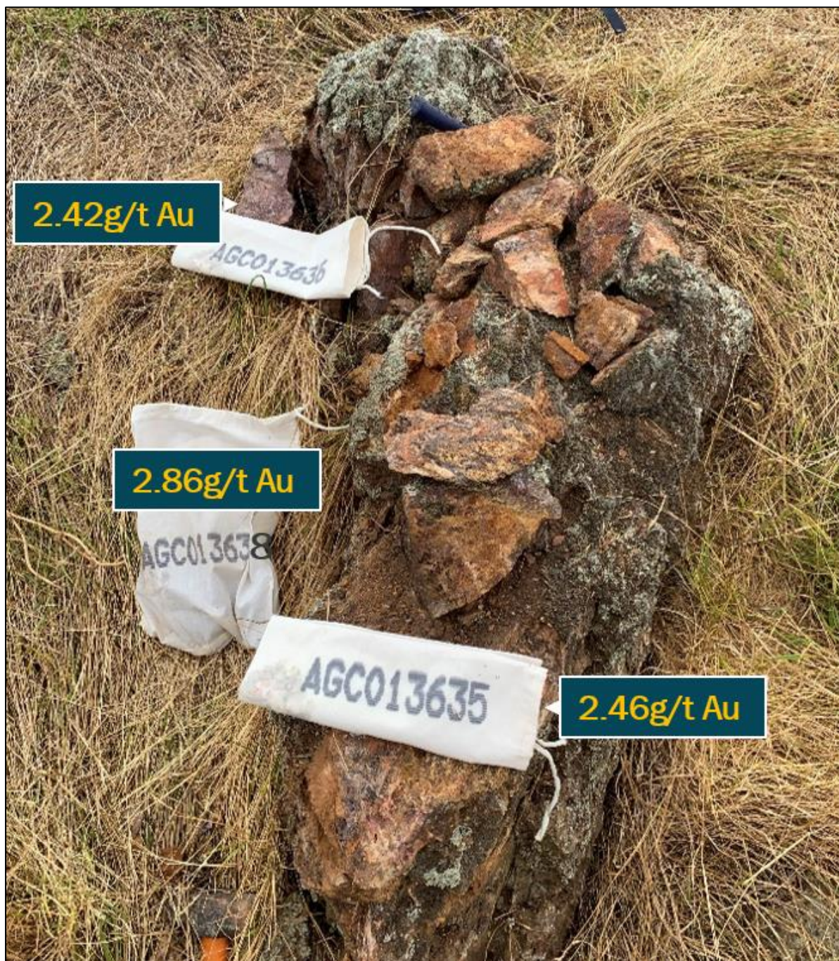
Figure 4: Rock chip sample sites AGC013635 – AGC013636 and AGC013638 showing gold results in the abundant gossanous (weathered sulphide) outcrop.
