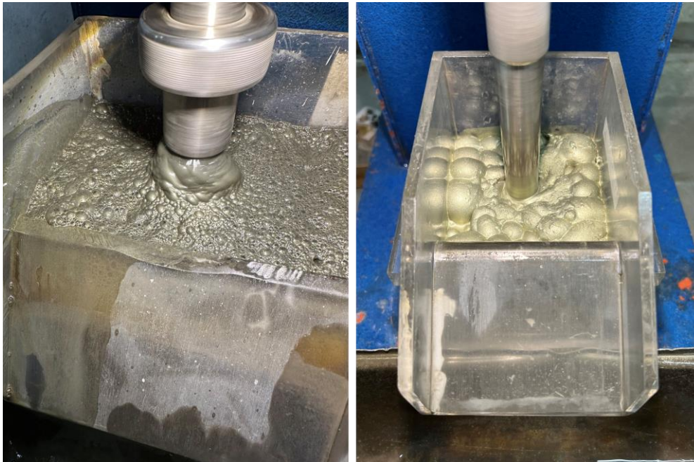
Figure 4. Photographs showing desktop rougher (left) and cleaner (right) froth flotation test work on a mineralised composite from the Corvette Prospect conducted by ALS Metallurgy in Burnie, Tasmania.
