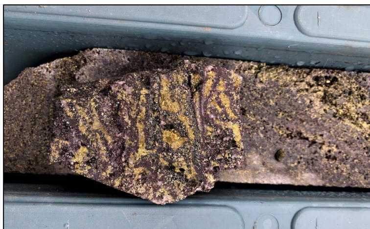
Photo 3. Chalcopyrite-specularite-hematite-magnetite mineralisation – SMD182, 423.5m drill depth, HQ3 diameter ½ cut drill core.
