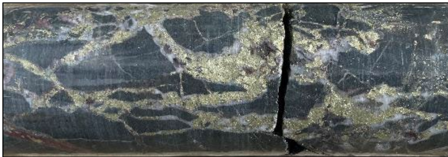
Photo 2. Chalcopyrite-quartz-hematite fill jigsaw breccia in chlorite-silica altered microdiorite - SMD173, 390.6m drill depth, HQ diameter uncut drill core. Note the dominance of chalcopyrite and hematite and the almost total lack of pyrite.
