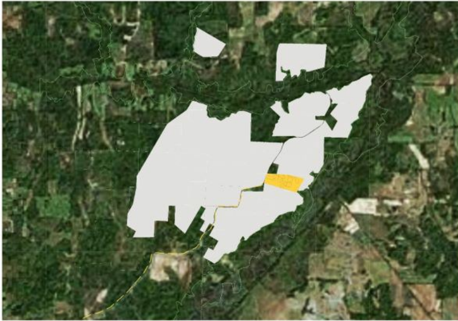
Figure 14: Titan Project mining outline (the mining outline defines the area mined and not a final open pit void as the process is incremental and pits are backfilled progressively)
