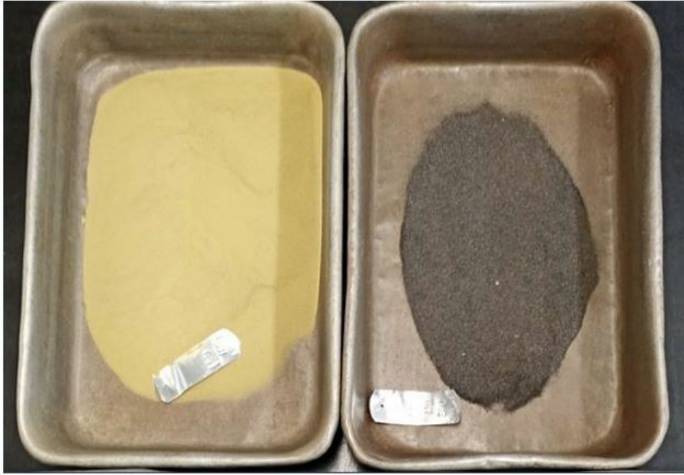
Figure 6: Rare earth (LHS) and heavy mineral concentrate (RHS) streams from wet shaking table tests after flotation.
