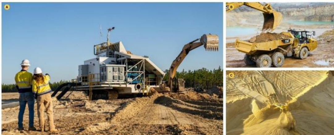
Figure 12: A – Example mobile mining unit mineralized material feed (courtesy of Mineral Technologies); B – Example dry mining of waste; C – Example wet sand tails waste.
