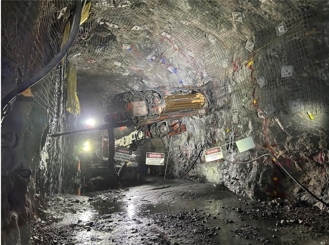
**Figure 2** – Long-hole stope drilling on 1280mRL level at Abra (Photo 19 May)
