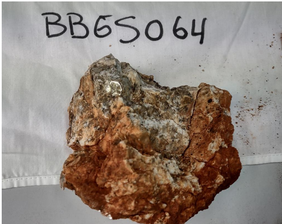
Figure 1: Samples of pegmatite BBGS050 (297044 mE, 6568534 mN, MGA94 Zone 51) and BBGS064 (298605 mE, 6581179 mN, MGA94 Zone 51) each with feldspar, mica, quartz and garnets.
