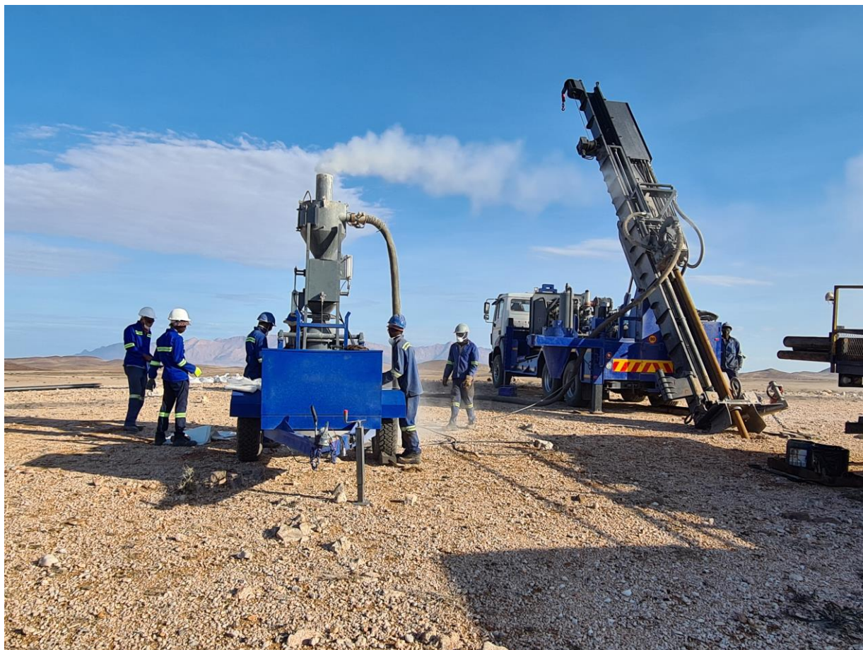
Figure 4: RC drilling rig operating during the second phase of RC drilling on EPL 7345.
