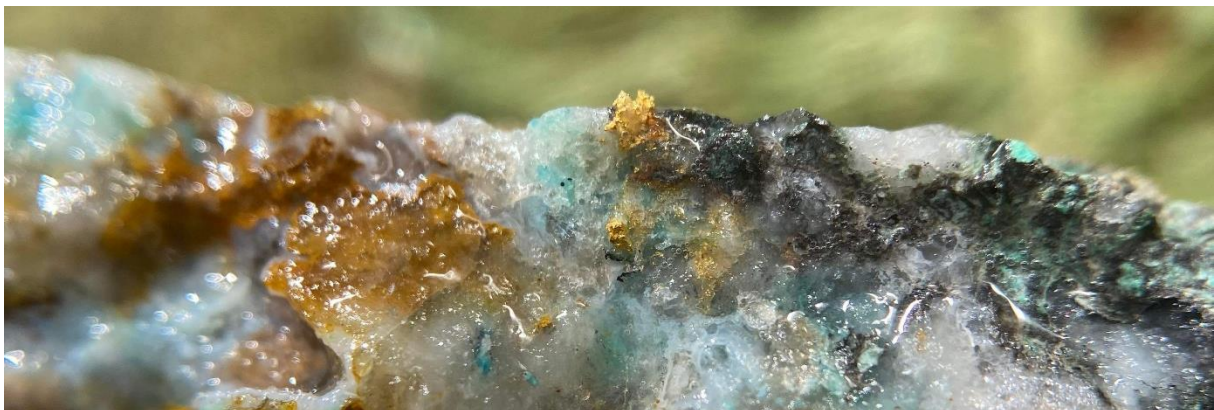
Figure 4: Image of visible gold within a quartz vein with secondary oxides and carbonates after sulphides from a mullock sample at the Lead Gold Mine (M09/091).
