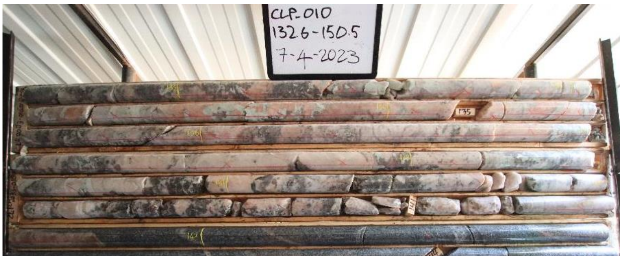
Photo 4: Chubb diamond drill hole CLP010 intercepted 8.25m at 1.31% Li 2 O from 130.45m displaying large crystal structure of the spodumene-bearing pegmatites.
