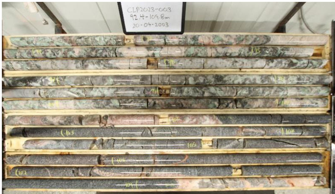
Photo 3: Chubb diamond drill hole CLP003 intercepted 12.22 m of large crystal structure of the spodumene-bearing pegmatites from 90.00m depth with an estimated 10 to 30% spodumene content.
