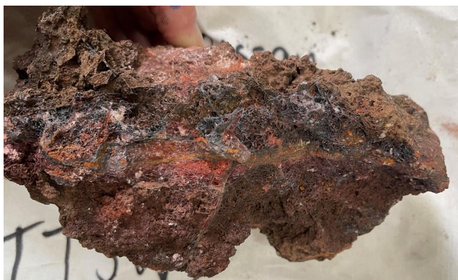
Figure 3. (above left) Sample QR59 with assays of 6.1% Cu and 0.5 % Zn; (above right) photo of outcrop of trench where samples were taken at Tea Tree north (see Table 1); (left) Sample TTSW2 with assays results of 6.9 g/t Au, 110 g/t Ag, 0.5% Cu from Tea Tree North
