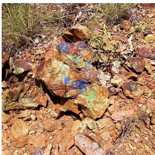
Figure 3. (above left) Sample QR59 with assays of 6.1% Cu and 0.5 % Zn; (above right) photo of outcrop of trench where samples were taken at Tea Tree north (see Table 1); (left) Sample TTSW2 with assays results of 6.9 g/t Au, 110 g/t Ag, 0.5% Cu from Tea Tree North
