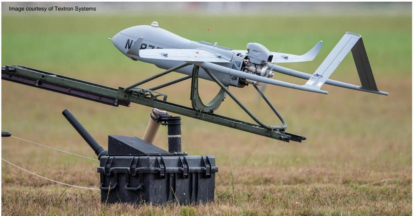
Orbital UAV has been contracted for the development of upgrades to engines for Textron Systems' Aerosonde<sup>®</sup> UAS.
