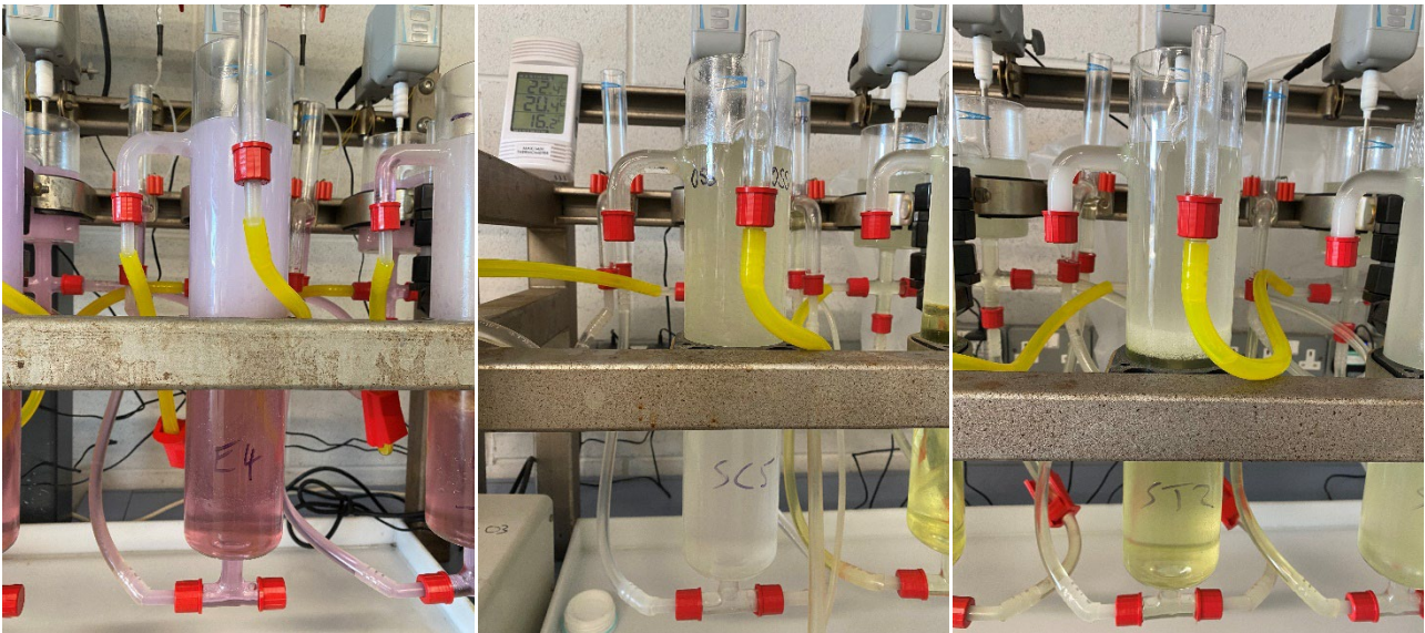
Figure 5: Pilot plant activities showing separation of neodymium (Nd) away from dysprosium (Dy), across extraction (left), scrubbing (centre) and stripping (right).
