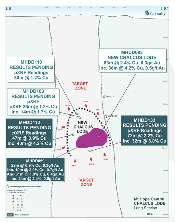
Figure 1. Mount Hope Central Chalcus Lode Long Section Showing New Drill Results.
