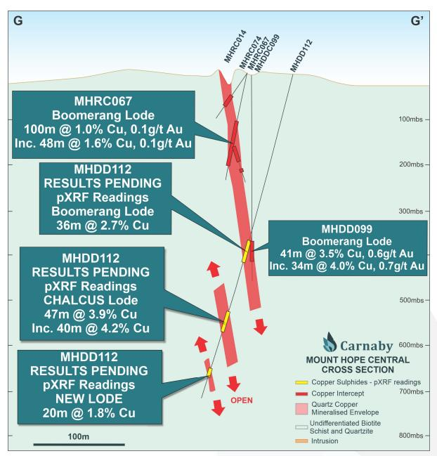
Figure 2. Mount Hope Central Drill Cross Section Showing New Results.
