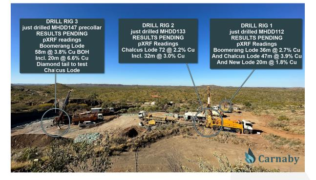
Figure 3. Photo of the three currently operating drill rigs looking northeast and labelled with pXRF readings from each of the last holes just completed by each rig.
