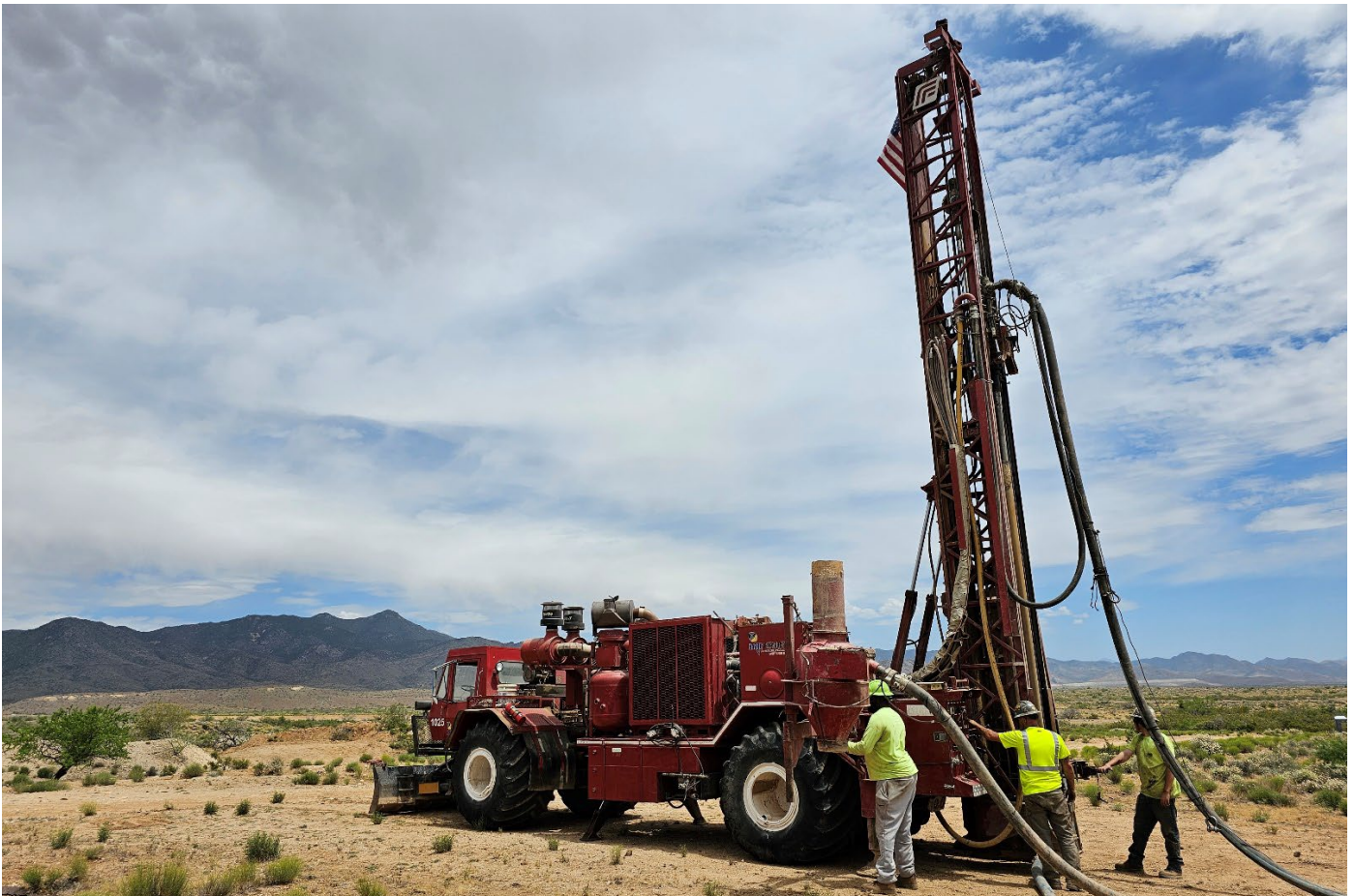
Figure 1: Harris Exploration reverse circulation drill rig at Riedel's Tintic prospect.
