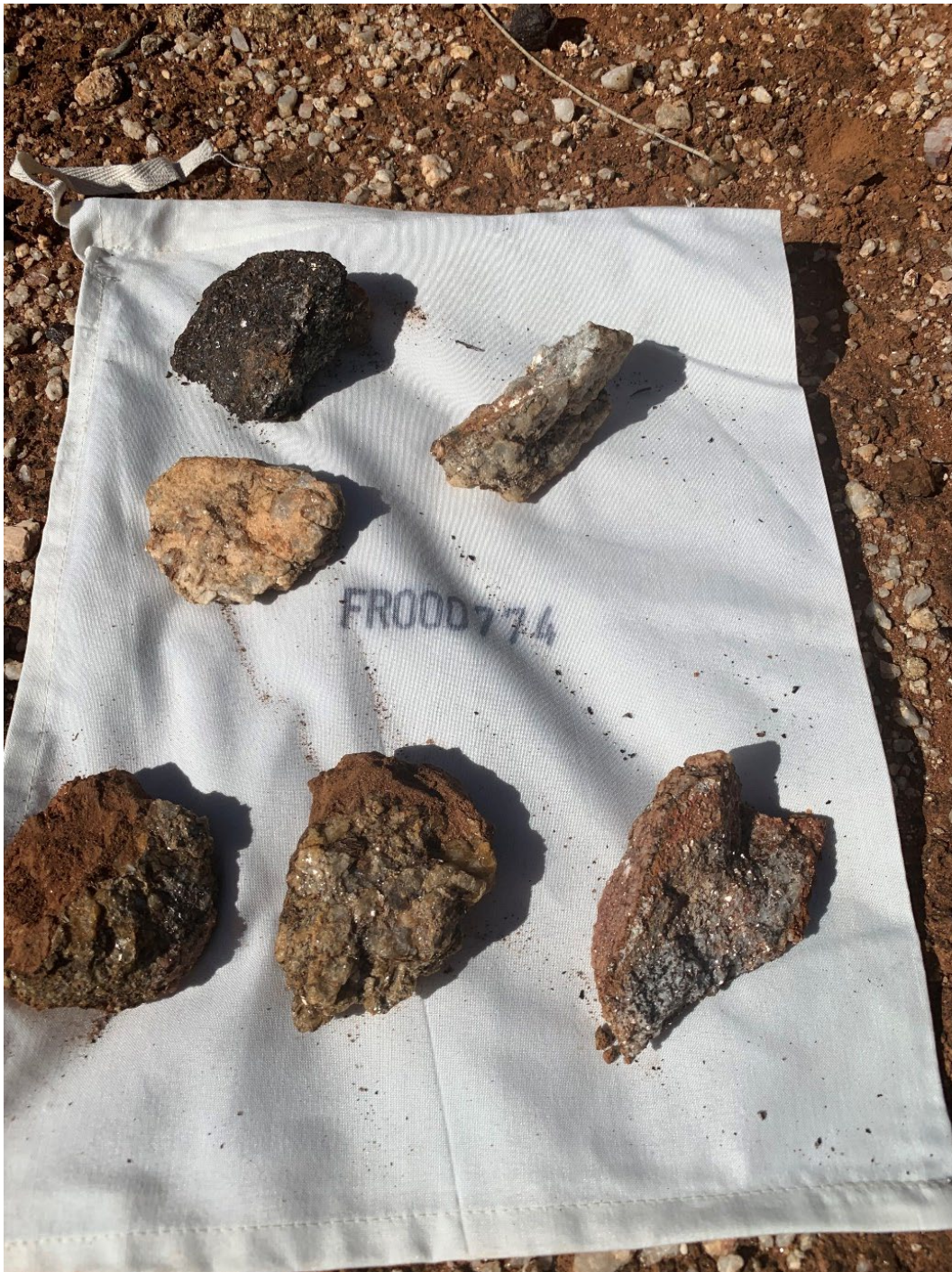
Figure 6: The Alexandra Bore/Breakaway Dam project area with muscovite bearing pegmatite sample, taken from the outcropping pegmatite in the previous image (Figure 5). Assay pending.
