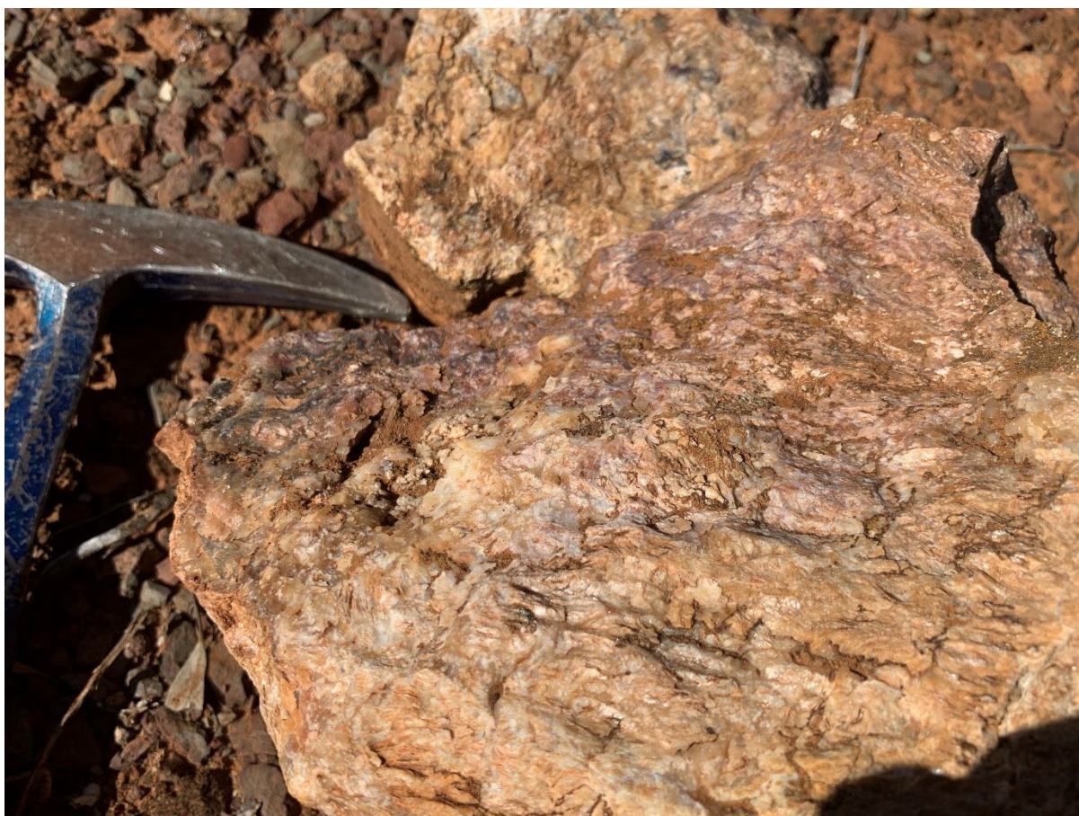
Figure 10: The Bonnie Vale project area with muscovite bearing, outcropping pegmatite sample, taken from the pegmatite outcrop in the previous image (Figure 9) – mapping/sample point FR000714. Assay pending.
